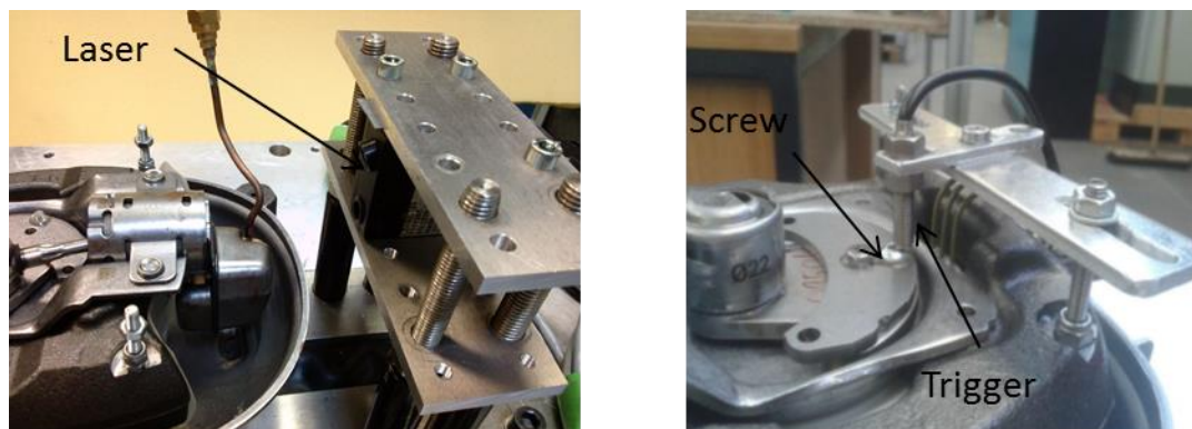
Figure 4: Left: Position of the laser in front of the suction valve. Right: Induction trigger used in combination with a screw for determining top dead center.
