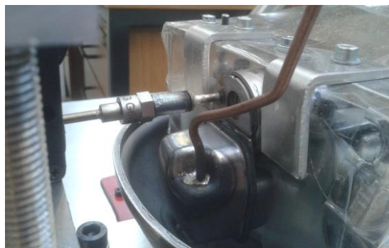
Figure 5: Pressure sensor mounted on the valve plate
