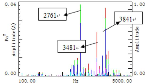
Figure 6: Frequency spectrums near compressor main body
