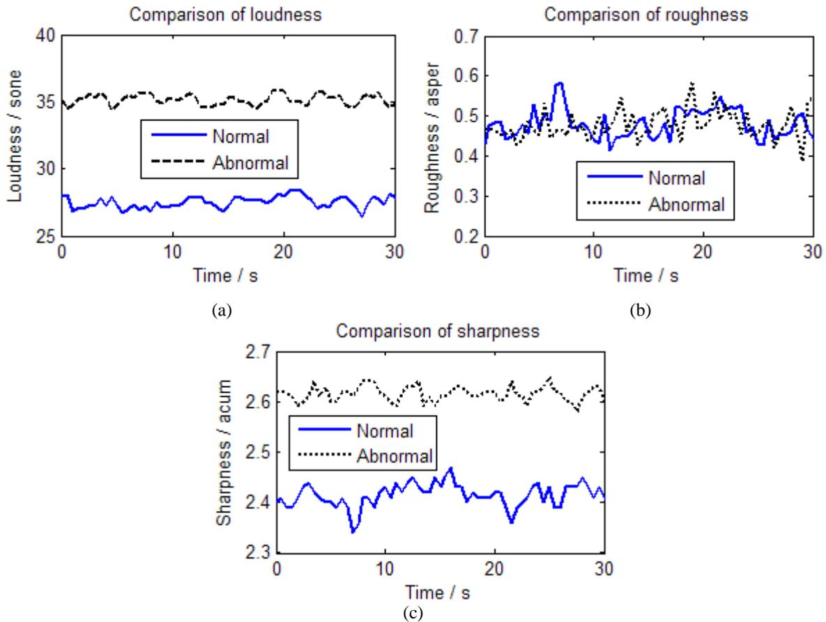
Figure 1: Objective evaluation parameters comparison of two compressors
