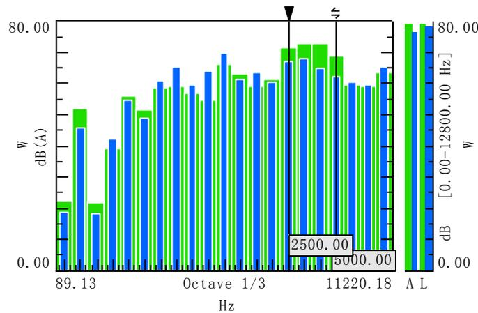
Figure 5: 1/3 octave spectrum comparison of two compressors
