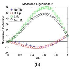
FIG. 8. (Color online) Experimentally measured ODSs of qPlus sensors. The tip displacement has been scaled to equal unity, the length has been normalized by the length of the beam. R tip denotes regular tip, L tip denotes long tip, XL tip denotes extra long tip. See Fig. 7 for photographs of the corresponding probes and tips and Tables I and II for geometrical details.
