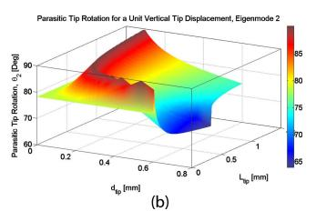
FIG. 4. (Color online) Surface plot of the angle of the tip, or parasitic tip rotation, calculated for a unit vertical tip displacement. (a) Parasitic tip rotation due to bending of the first eigenmode, for a unit vertical tip displacement. (b) Parasitic tip rotation due to bending of the second eigenmode, for a unit vertical tip displacement. Note that at the critical tip length when the tip becomes a node of vibration the tip motion is dominated by the parasitic tip rotation.
