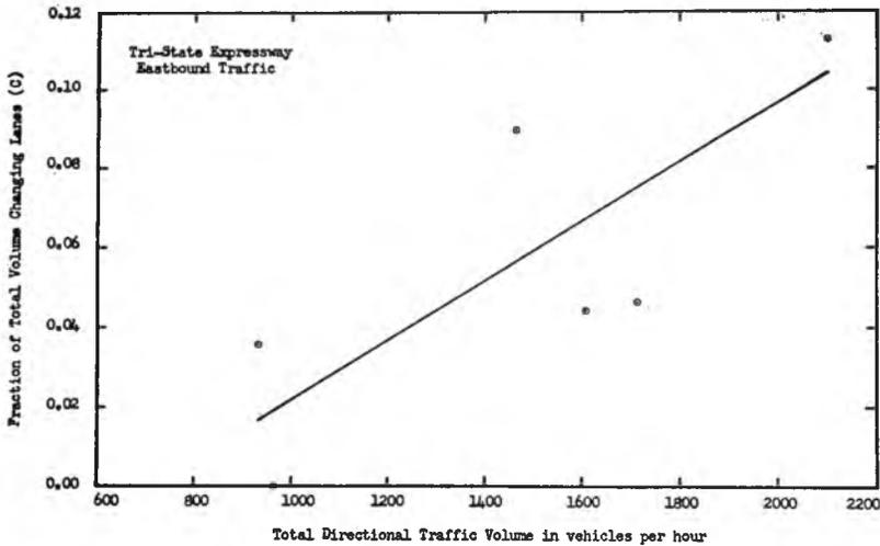
Fig. 18. Lane changing as a function of directional volume on a four-lane freeway as measured on aerial photographs.
