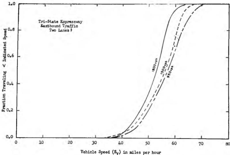
**Fig. 8. Vehicle speed distribution at various directional traffic volumes on a four-lane freeway as measured on aerial photographs.**
