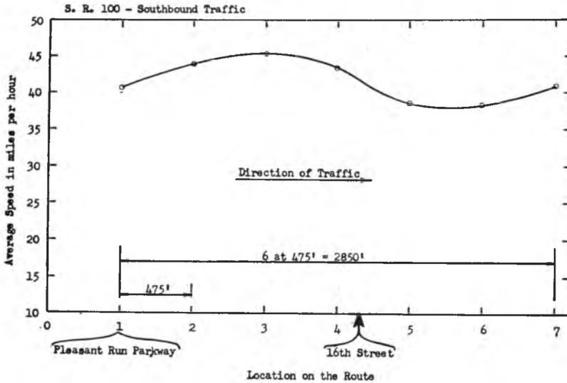
Fig. 16. Average vehicle speed for directional traffic as a function of the location on the route as measured on aerial photographs.
