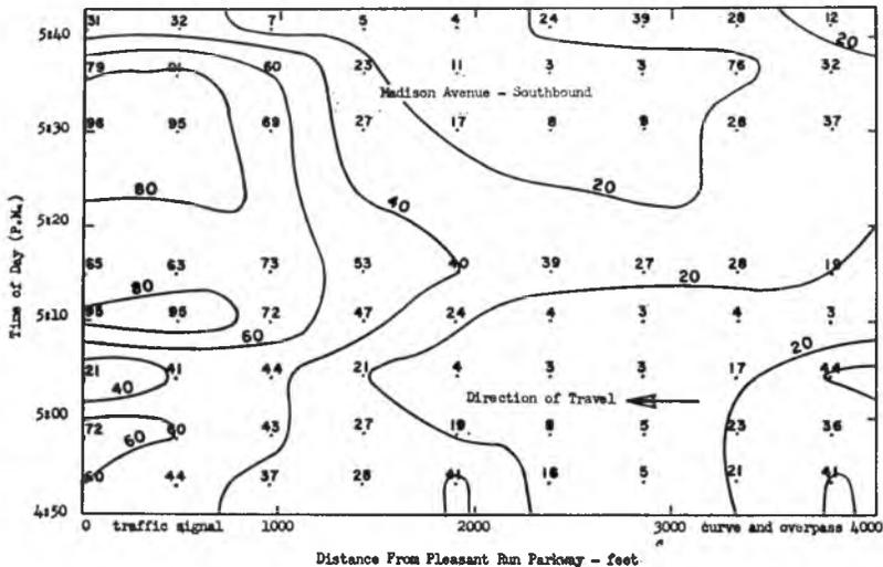
Fig. 12. Traffic density contour map prepared from aerial photographs.
