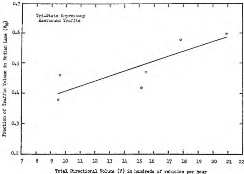
Fig. 11. Fraction of the directional traffic volume in the median lane at various volumes on a four-lane freeway as measured on aerial photographs.
