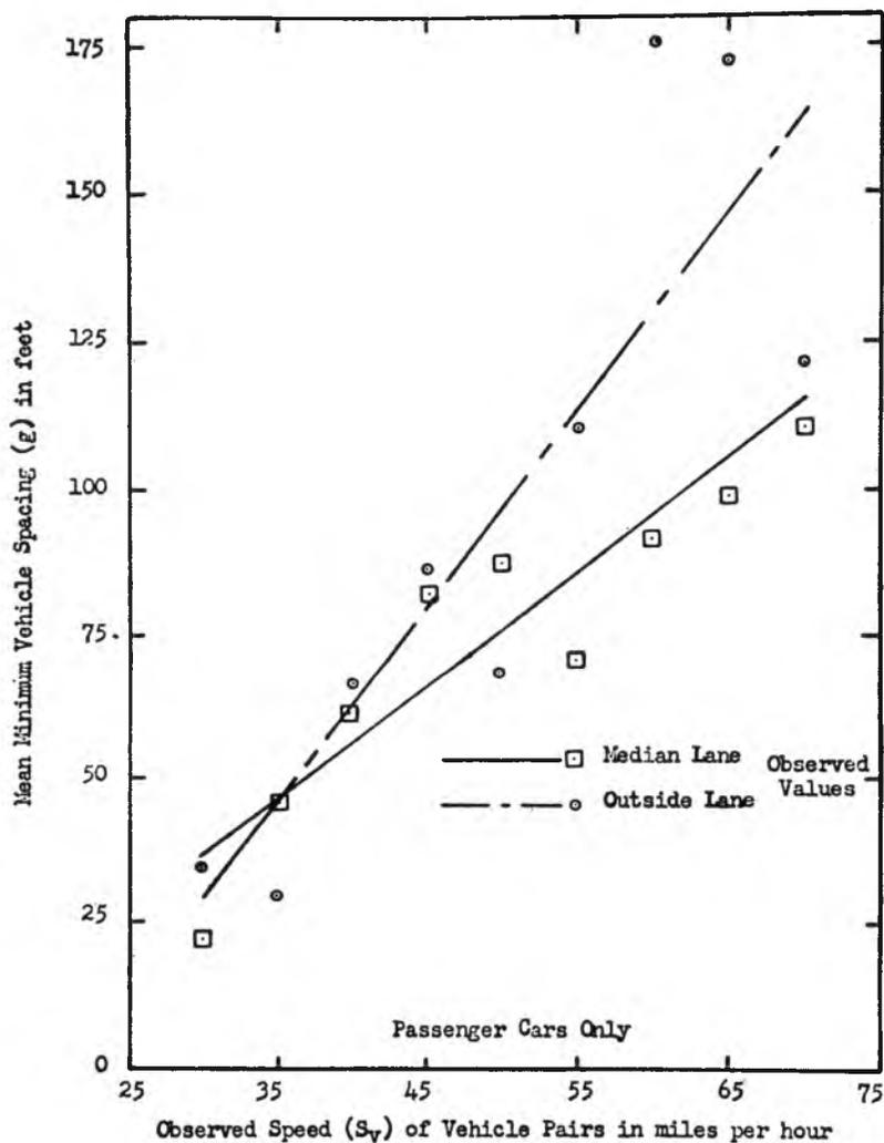
Fig. 17. Minimum spacings allowed by the average driver when trailing another vehicle at various speeds on four-lane divided highways as measured on aerial photographs.
