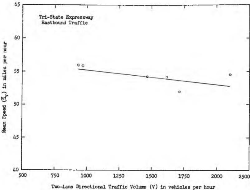
Fig. 9. Mean speed as a function of directional traffic volume on a four-lane freeway as measured on aerial photographs.
