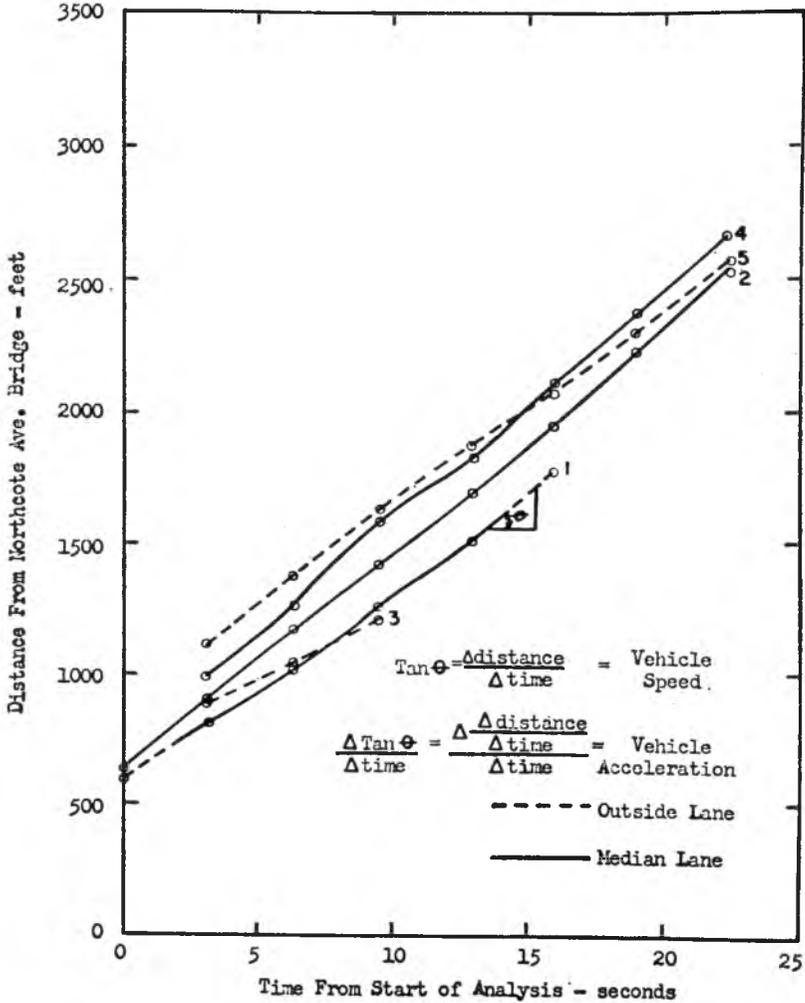
Fig. 15. Tracking the movement of individual vehicles in time and space by the use of aerial photography.
