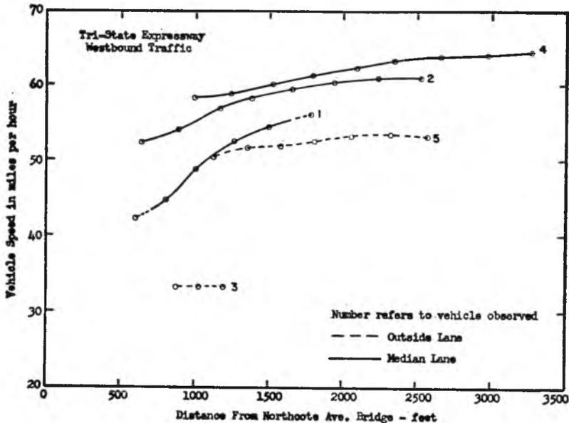
Fig. 14. Vehicle acceleration and speed patterns on a four-lane freeway as measured on aerial photographs.
