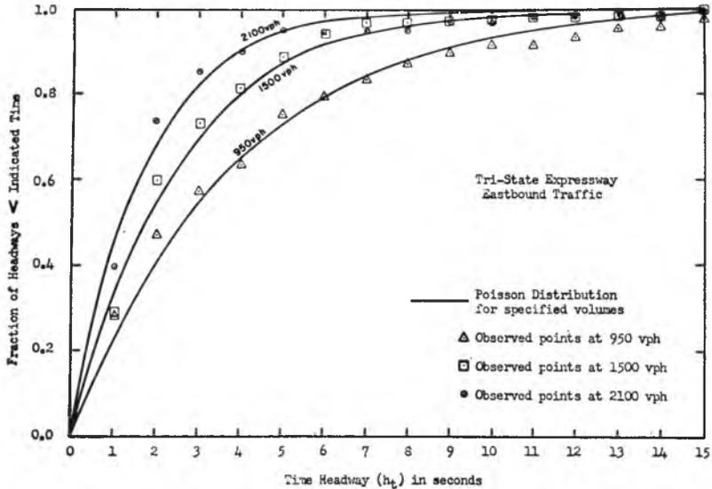
Fig. 10. Cumulative frequency distribution of vehicle time headways at various directional volumes on a four-lane freeway as measured on aerial photographs.
