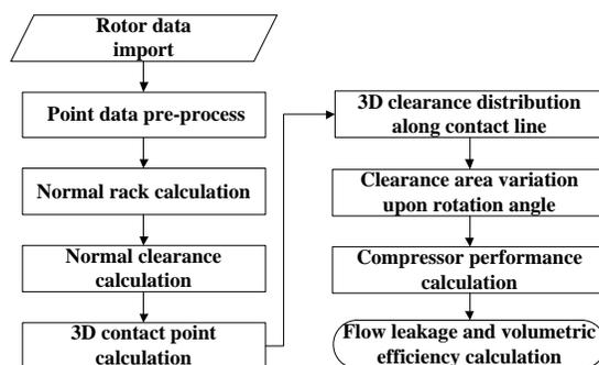
**Figure 2:** Flowchart of normal clearance calculations
