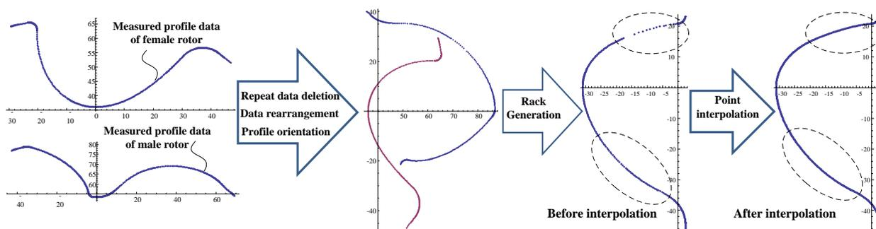
**Figure 3:** Point data pre-process and interpolation
