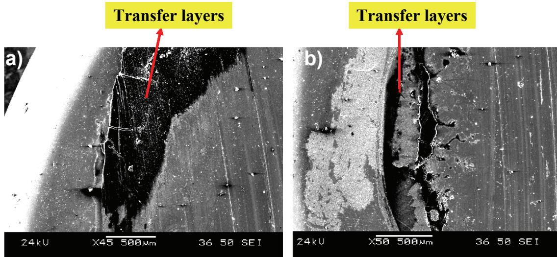
Figure 4: SEM images of the 52100 steel shoes tested against PTFE/MoS<sub>2</sub> where (a) and (b) show two different regions on the surface of the 52100 steel pin.
