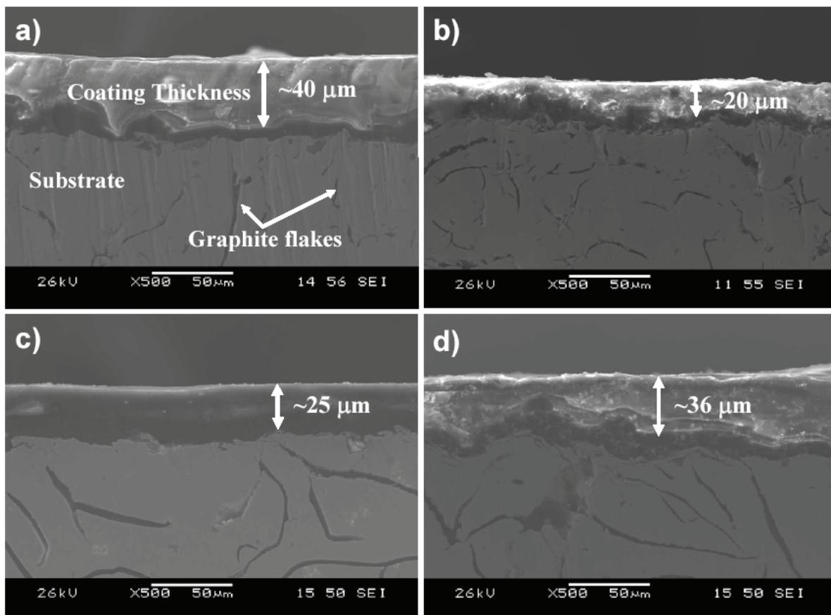
Figure 2: Cross section SEM images of the different coated disks. a) PEEK/PTFE, b) PTFE/MoS<sub>2</sub>, c) Fluorocarbon, d) PEEK/PTFE/Ceramic.
