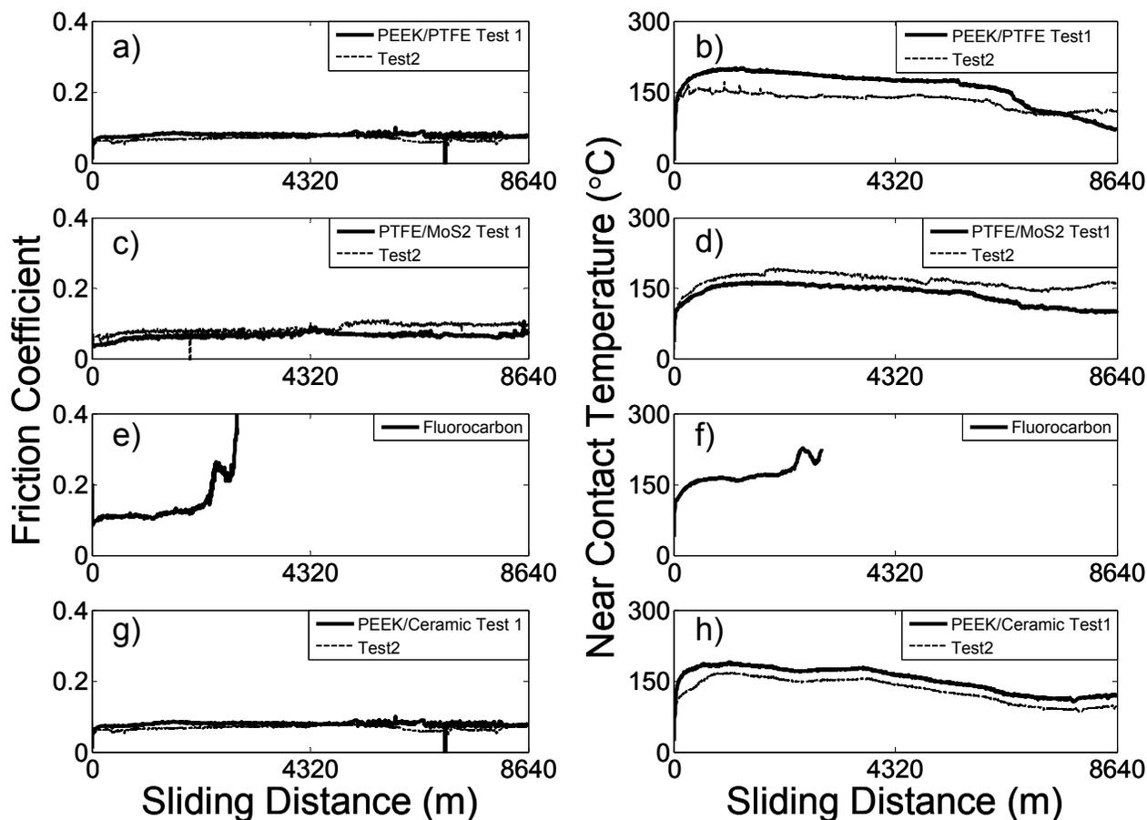
Figure 3: Typical experimental results depicting friction coefficient and near contact temperature for (a), (b) PEEK/PTFE, (c), (d) PTFE/MoS<sub>2</sub>, (e), (f) Fluorocarbon, and (g), (h) PEEK/PTFE/Ceramic.
