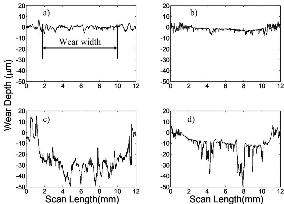
Figure 5: Profilometric wear measurements, (a) PEEK/PTFE, (b) PTFE/MoS<sub>2</sub>, (c) Fluorocarbon, and (d) PEEK/PTFE/Ceramic.
