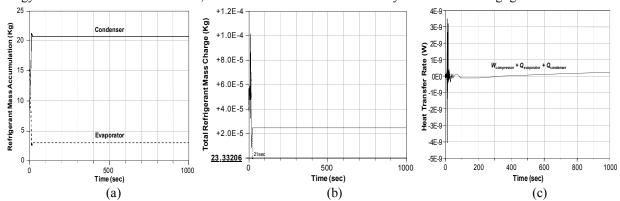
Figure 3: (a) is the refrigerant movement during start-up and steady state mass accumulation in the condenser and evaporator, respectively, (b) is the total refrigerant mass charge in the chiller cycle (check of mass conservation) and (c) is the total refrigerant energy balance in the chiller cycle (check of energy conservation)
