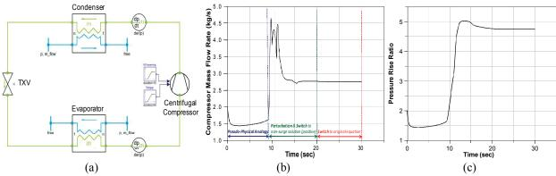
Figure 2: Simulation study of the proposed initialization method where (a) is the Dymola layout of the centrifugal chiller model, (b) is the mass flow rate at compressor outlet during the initialization phase and (c) is the pressure rise ratio during the initialization phase
