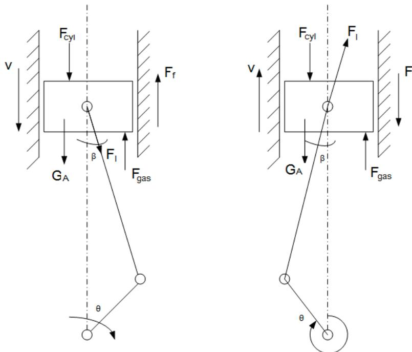
Figure 1: Force and moment analysis of the crank-connecting rod system
