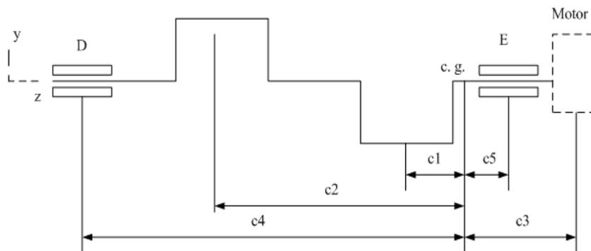
Figure 3: Crankshaft illustrations with dimensions
