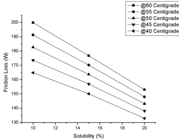
Figure 4: Solubility-Friction loss relation at different temperatures
