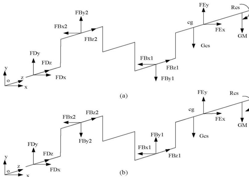
Figure 2: Force and moment analysis of the crankshaft
