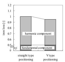
Figure 11 – Iron loss of magnet positioning
