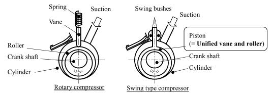
Figure 1 - Mechanism of rotary and swing type compressor
