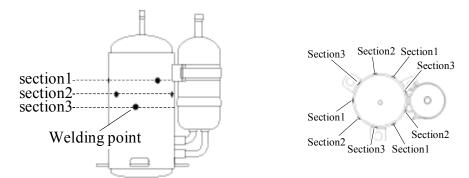
The exterior view of the developed compressor
