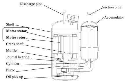
Figure 2 – Cross sectional view of swing type compressor
