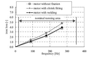
Figure 5 – Iron loss of motor stator fixation method
