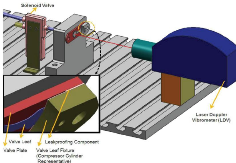
Fig. 1. Schematic display of the test system
