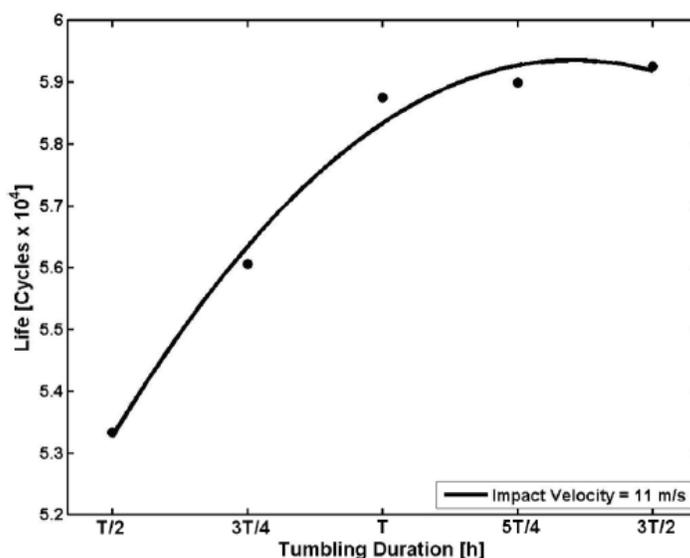
Fig. 3. The effect of tumbling duration on impact fatigue life of carbon strip steel.
