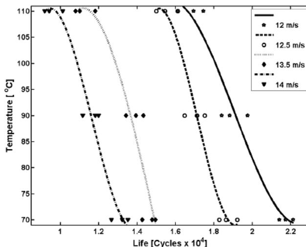
Fig.7. The influence of temperature on the impact fatigue life of carbon strip steel.
