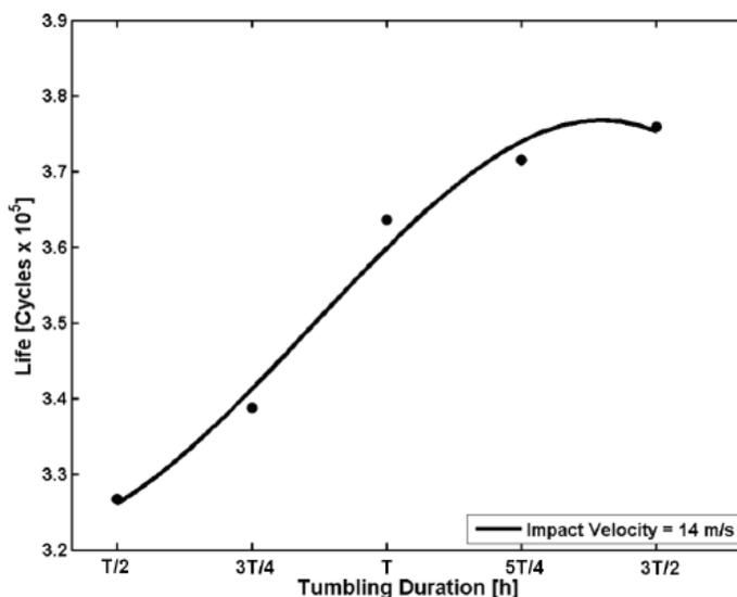
Fig. 4. The effect of tumbling duration on impact fatigue life of stainless strip steel.
