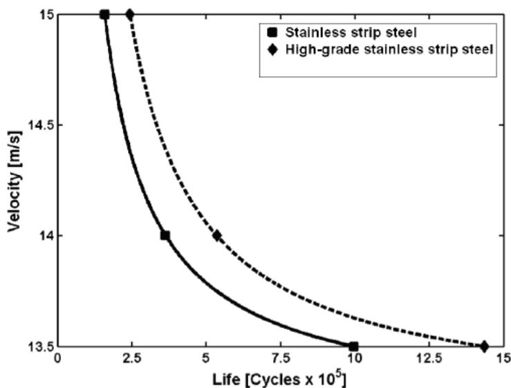
Fig. 6. Comparison of stainless strip steel and high-grade stainless strip steel.
