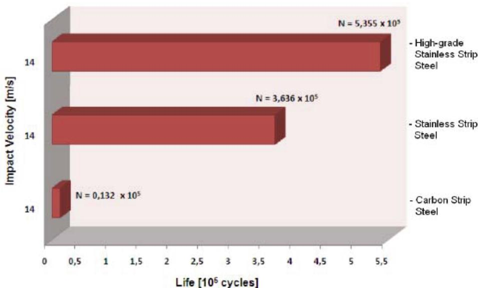
Fig. 5. Comparison of impact fatigue life for 14 m/s impact velocity
