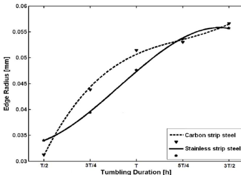
Fig. 2. Effect of the tumbling duration on the edge radius
