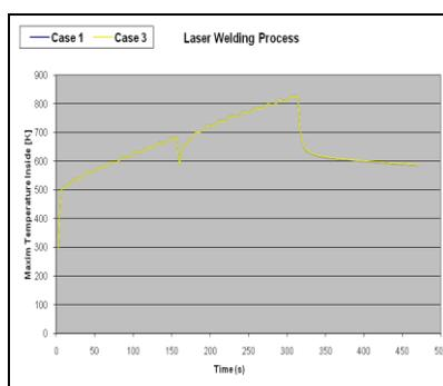
Figure 07 – Maximum inside temperatures through laser welding process.
