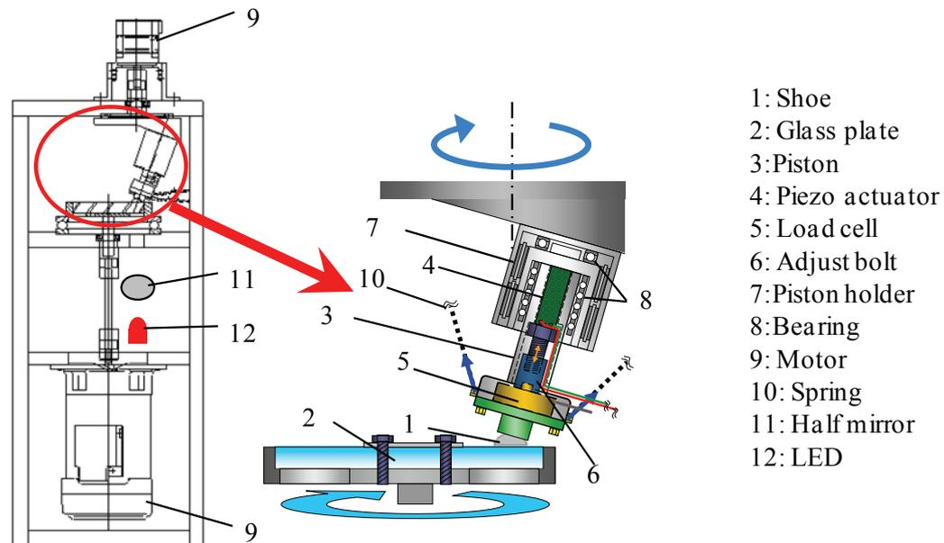
Figure 3 Schematic view of model experimental apparatus
