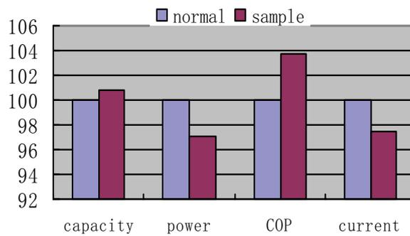
Fig.6 Chart of performance change on large volume compressor using nano-materials
