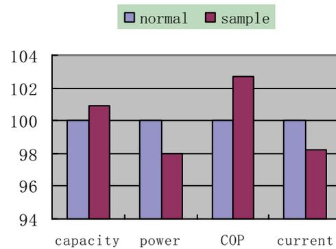
Fig.3 Chart of performance change before and after using nano-materials
