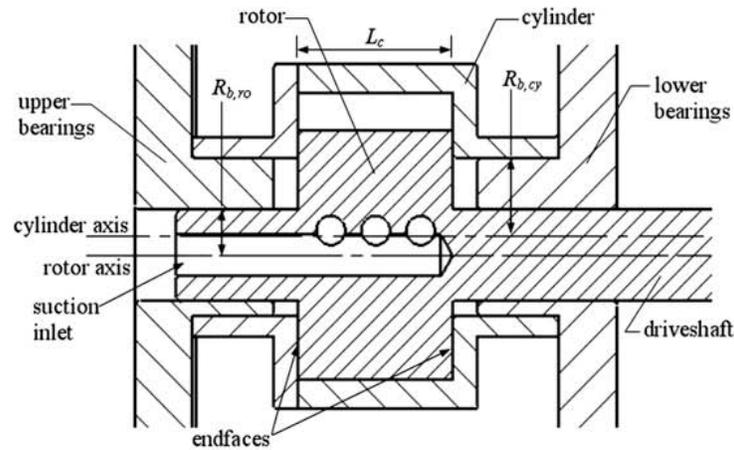
Figure 1: Side-view of the RV compressor (Teh and Ooi, 2009a)
