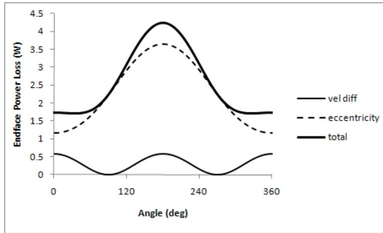
Figure 4: Endface power loss of a RV machine
