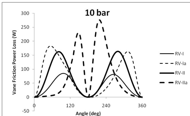
Figure 8: Vane side friction power losses of the four possible RV expander designs at 10 bar suction pressure
