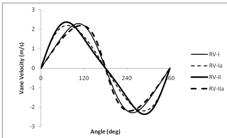
Figure 9: Vane sliding velocities of the four possible RV expander designs
