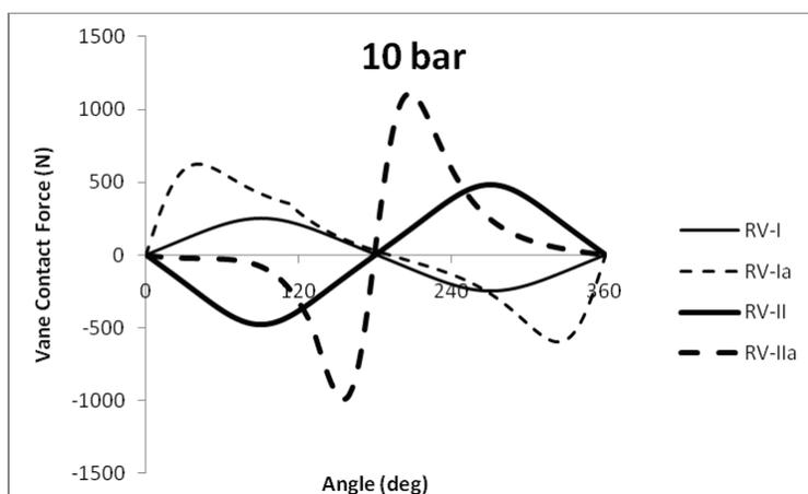
Figure 5: Vane contact forces of the four possible RV expander designs at 10 bar suction pressure
