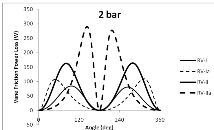
Figure 6: Vane side friction power losses of the four possible RV expander designs at 2 bar suction pressure
