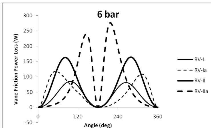
Figure 7: Vane side friction power losses of the four possible RV expander designs at 6 bar suction pressure
