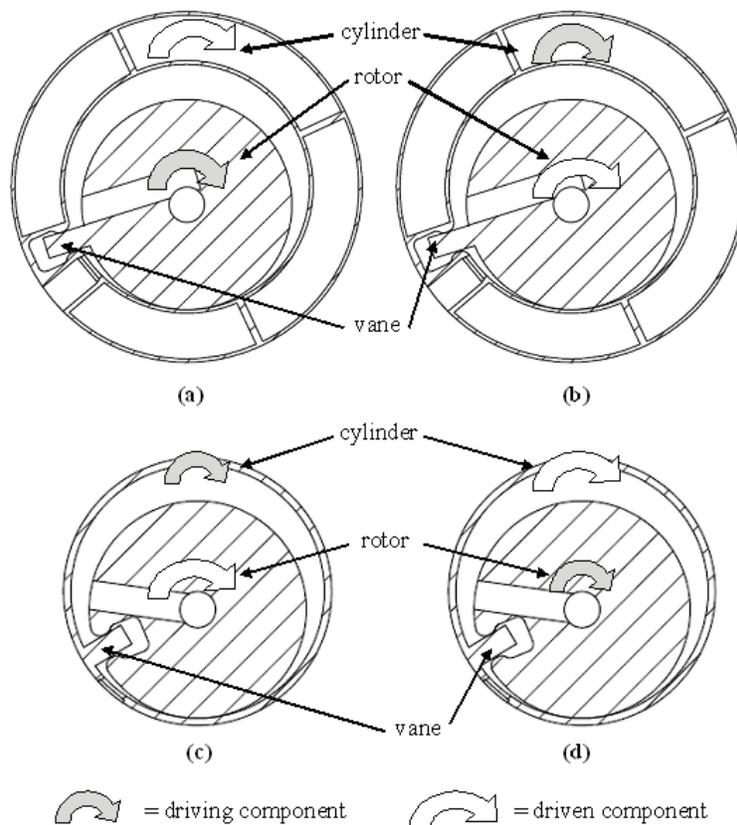
Figure 1: Alternative RV mechanism designs: (a) RV-I, (b) RV-Ia, (c) RV-II, (d) RV-IIa
