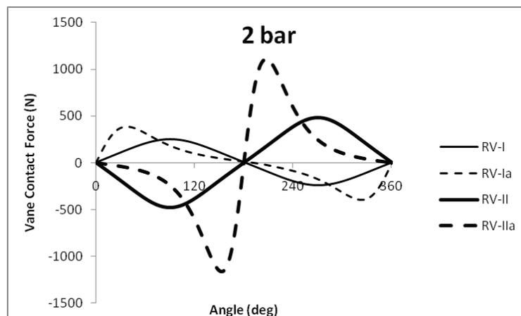
Figure 3: Vane contact forces of the four possible RV expander designs at 2 bar suction pressure
