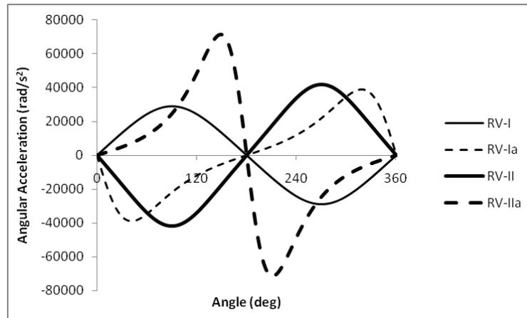
Figure 2: Angular accelerations of the driven components of the four possible RV expander designs
