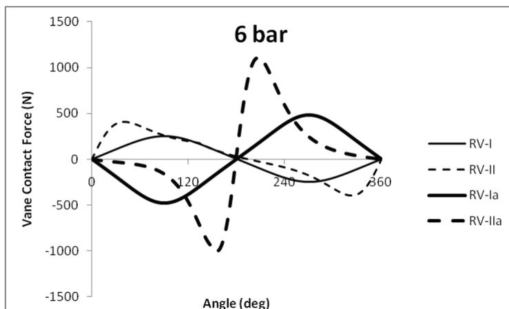
Figure 4: Vane contact forces of the four possible RV expander designs at 6 bar suction pressure
