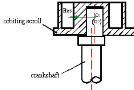
Fig.2 embedded-type-shaft scroll
