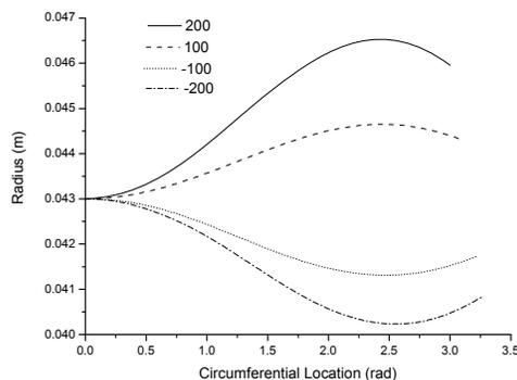
Figure 9 Free shape for different uniform tension distribution
