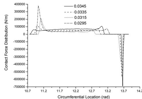
Figure 10 Contact for distribution under different constant radius
