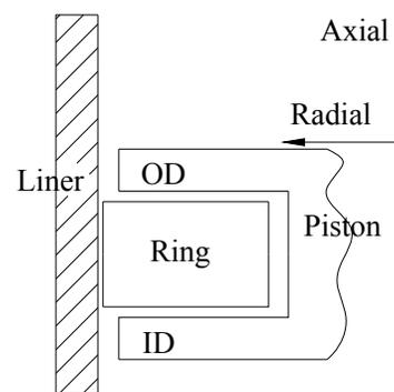
Figure 6 Cross-section of a piston ring
