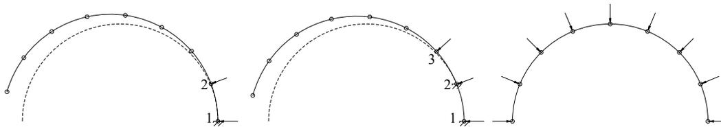
Figure 2 Step-by-step procedure of fitting a ring to a circular bore
