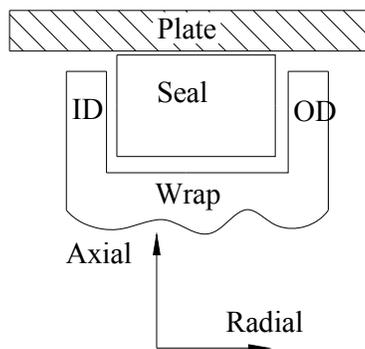
Figure 5 Cross-section of a tip seal
