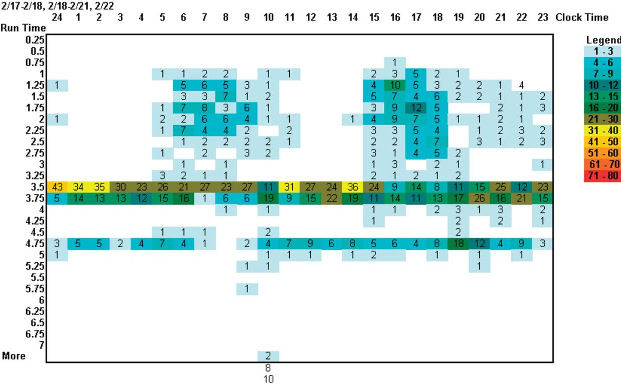
Figure 2 – Compressor Run Time Histogram
