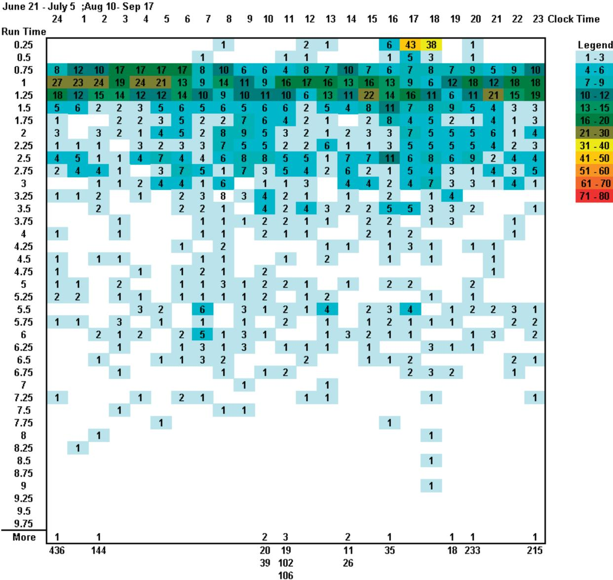
Figure 1 – Compressor Run Time Histogram Synchronous Operation
