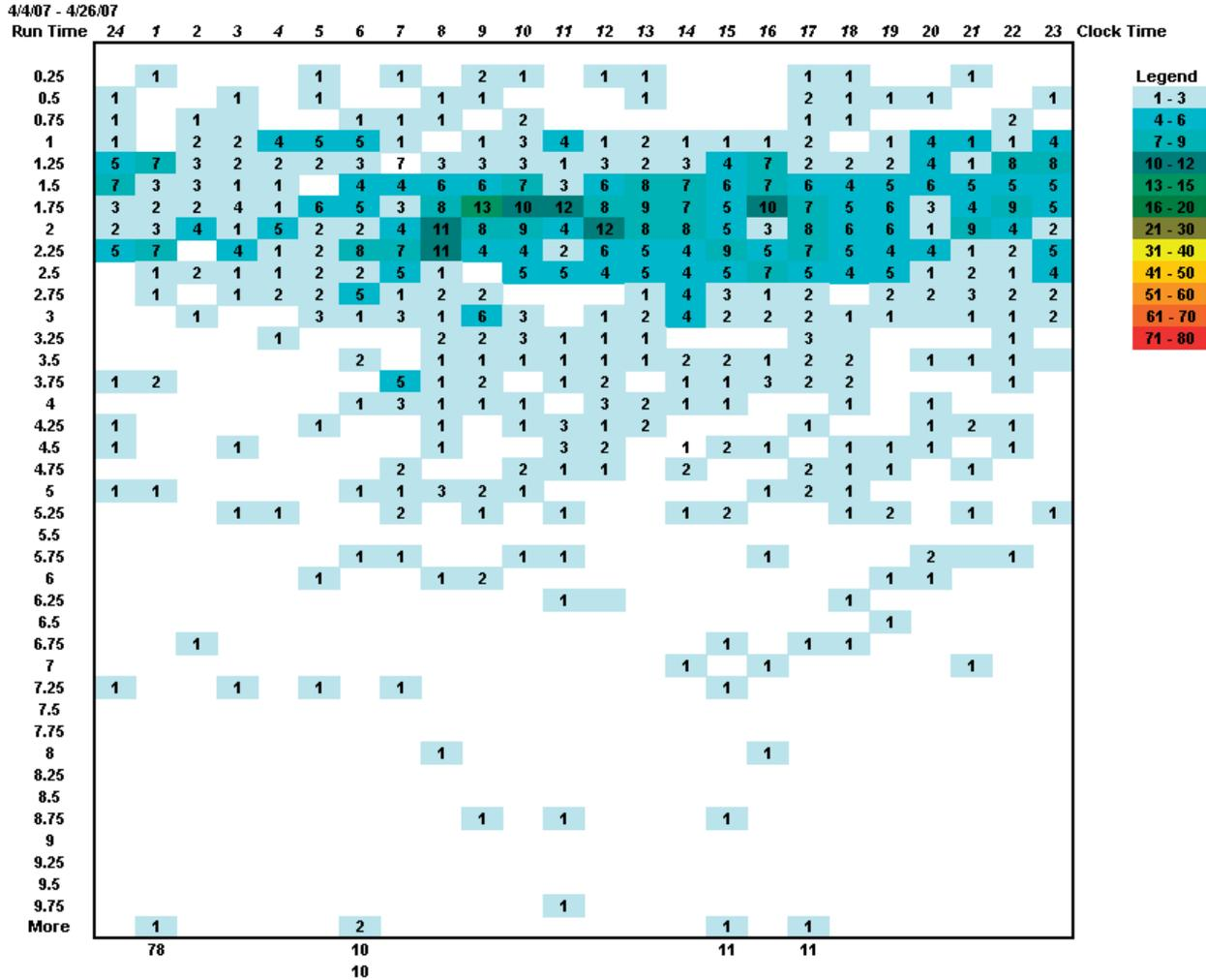
Figure 6 – Compressor Run Time Histogram
