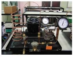
Figure 4.1: Durability test bench
