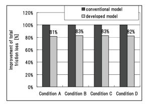
Fig.5: Improvement of friction loss
