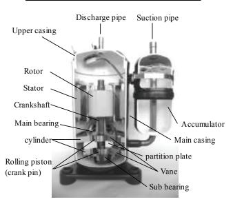
Fig.3: Cross section of developed compressor
