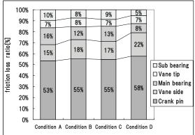
Fig.4: Friction loss ratio of conventional model
