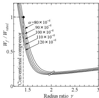
Figure 11 Non-dimensional energy loss  $W_f/W_{rated}$  ( $\Delta p=0.6$  MPa,  $N=3600$  rpm).
