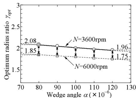
Figure 12 Optimum radius ratio  $\gamma_{opt}$  vs. wedge angle  $\alpha$  ( $\Delta p=0.6$  MPa).
