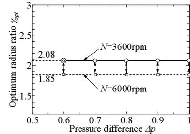
Fig. 15 Optimum radius ratio  $\gamma_{opt}$  vs. pressure difference  $\Delta p$ .
