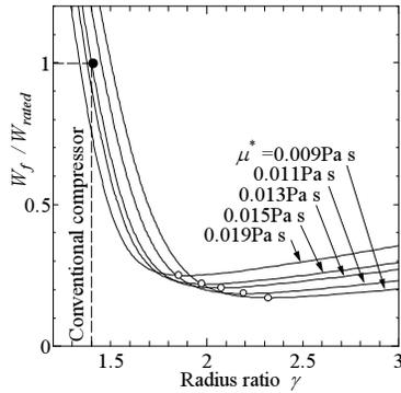
Figure 8 Non-dimensional energy loss  $W_f/W_{rated}$  ( $\Delta p=0.6$  MPa,  $N=3600$  rpm)
