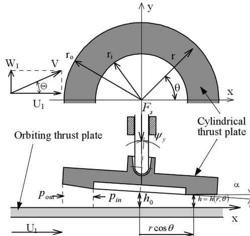
Figure 4 Mathematical model of thrust slide-bearing for theoretical analysis of fluid lubrication.
