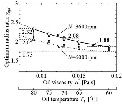
Figure 9 Optimum radius ratio  $\gamma_{opt}$  vs. oil viscosity  $\mu^*$  ( $\Delta p=0.6$  MPa).
