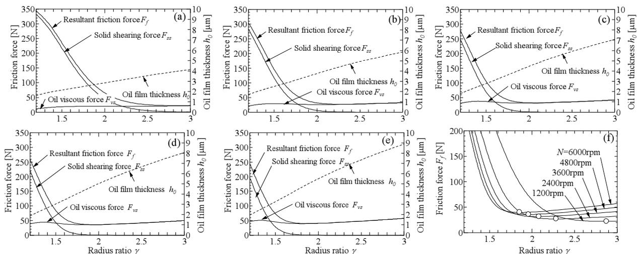
Figure 5 Calculated results of friction force  $F_{ss}$ ,  $F_{vs}$ ,  $F_f$  and oil film thickness  $h_0$  vs. radius ratio  $\gamma$  ( $\Delta p=0.6$  MPa):
