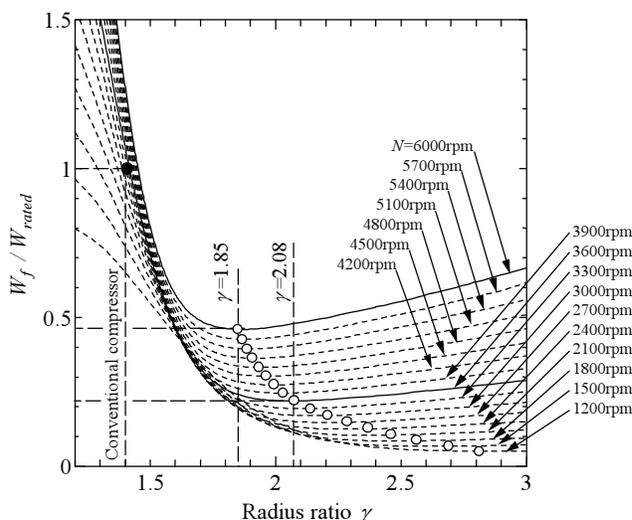
Figure 6 Non-dimensional energy loss  $W_f/W_{rated}$  ( $\Delta p=0.6$  MPa).
