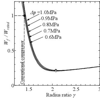
Fig. 14 Non-dimensional energy loss  $W_f / W_{rated}$  ( $N=3600$  rpm).
