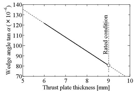
Figure 10 Wedge angle  $\alpha$  vs. thrust plate thickness.
