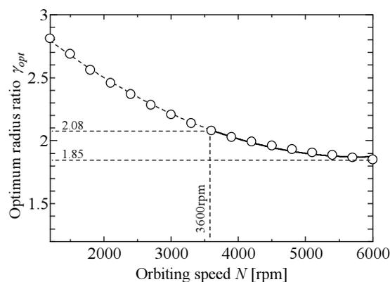
Figure 7 Optimum radius ratio  $\gamma_{opt}$  vs. orbiting speed  $N$  ( $\Delta p=0.6$  MPa).
