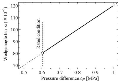
Fig. 13 FEM calculated wedge angle  $\alpha$  vs. pressure difference  $\Delta p$ .
