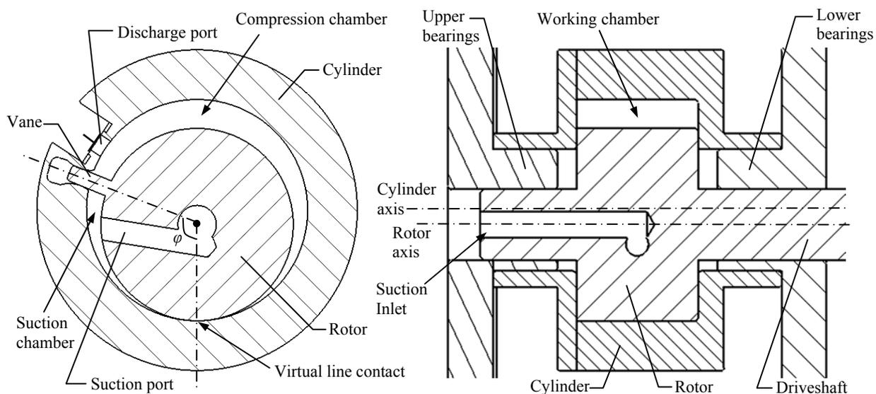
Figure 4: (Left) Front sectional view of RV-i compressor; (Right) Side sectional view of RV-i compressor with journal supports shown
