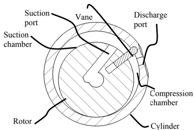
Figure 2 A schematic of a revolving vane compressor
