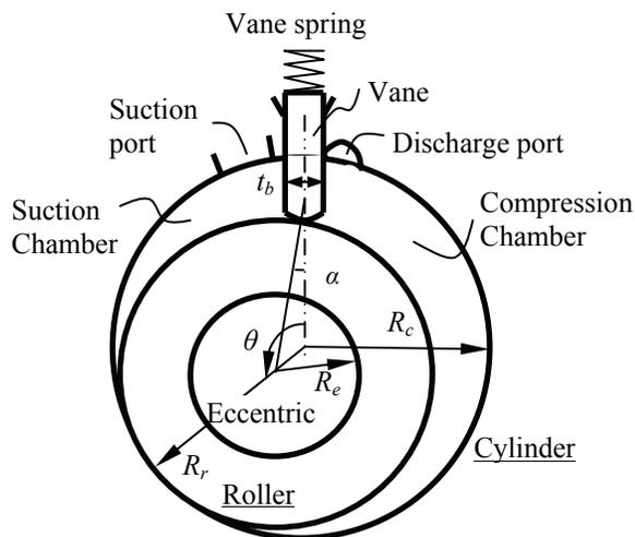
Figure 1 A schematic of a rolling piston compressor
