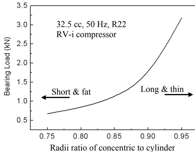
Figure 5: Variations of bearing forces for various geometrical configurations
