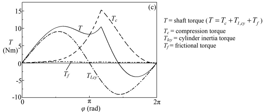
Figure 3: Variation of shaft torque and its components for revolving vane compressor: ( $T_c$  also represents the typical qualitative shaft torque in rolling piston compressors.)
