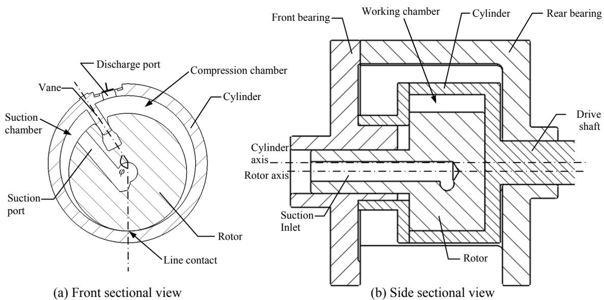
Figure 6: Sectional views of RV-i compressor with the vane fixed on the cylinder. It is better to directly drive the cylinder in this case.
