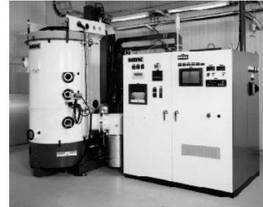
Fig. 15 The processing equipment of DLC-Si (A product made in NDK, Incorporated)
