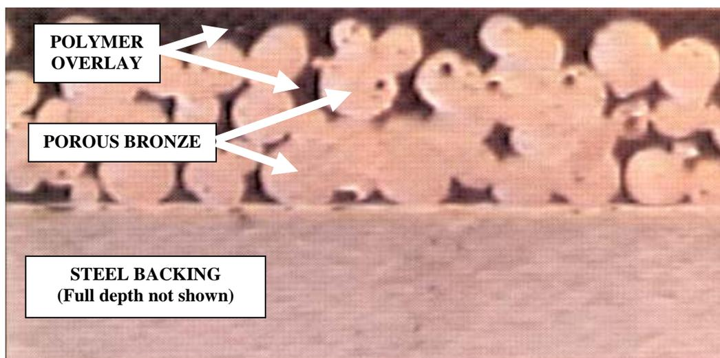
Figure 1: Cross-section of typical metal-polymer bushings
