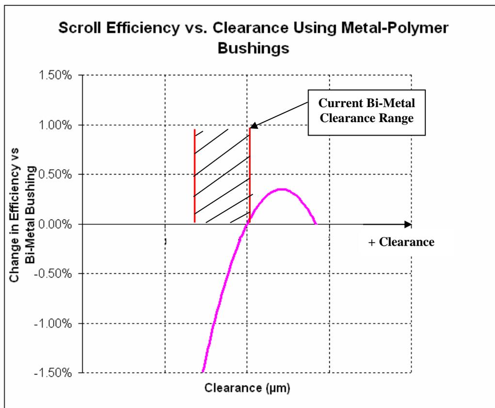
Figure 3: Metal-polymer efficiency vs. bi-metal efficiency over a particular clearance range
