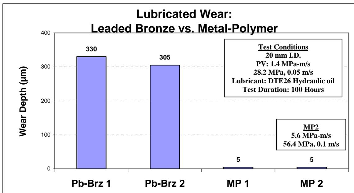
Figure 2: Lubricated wear of leaded bronze vs. metal-polymer bushings with test conditions
