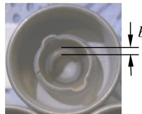
Figure 3.4 Band on the ball seat
