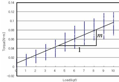
Figure 4.1 Relation between applied forces and friction torques
