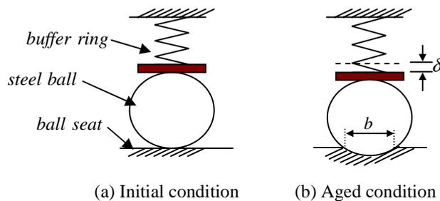
Figure 2.3 Ball joint configurations before and after the aging
