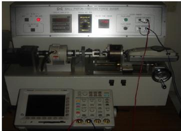
Figure 3.1 Friction torque-meter
