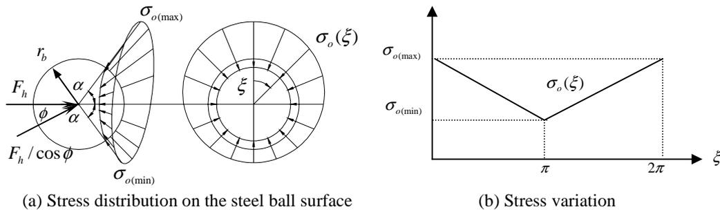
Figure 2.2 Stress distribution on the ball surface
