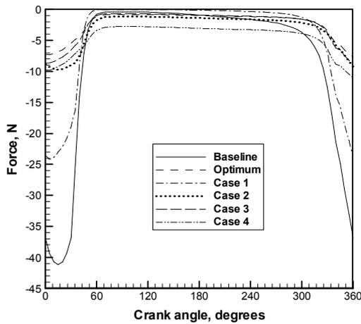
Figure 8 Boundary contact forces for optimized cases
