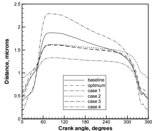
Figure 6 Minimum film thickness for improved cases
