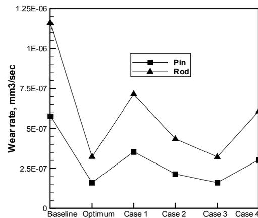
Figure 9 Cycle averaged wear rates for optimized cases
