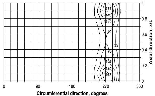
Figure 11 Accumulated wear rate of wristpin on the lubricated portion for the “optimum” case,  $\text{mm}^3/\text{s} \times 10^{12}$
