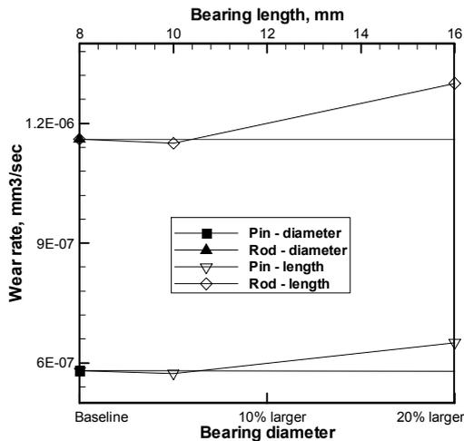
Figure 5 Effect of bearing diameter and length on cycle averaged wear rate
