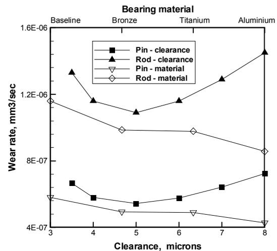
Figure 4. Effect of nominal clearance and pin material on cycle averaged wear rate
