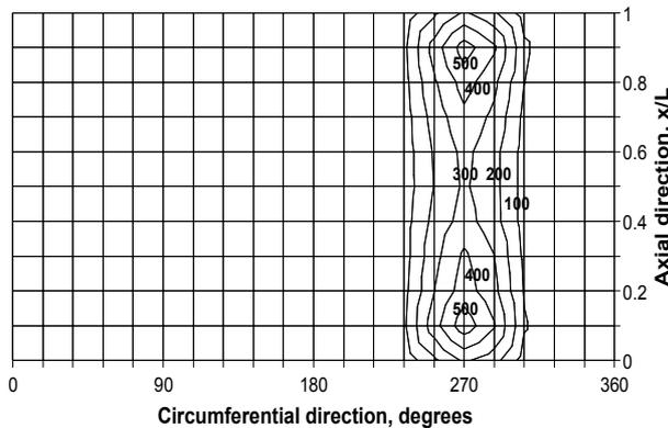
Figure 10 Accumulated wear rate of wristpin on the lubricated portion for the baseline case,  $\text{mm}^3/\text{s} \times 10^{12}$
