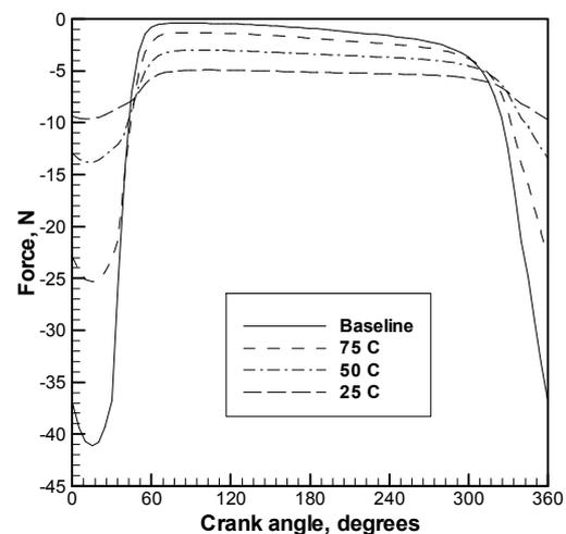
Figure 2. Effect of lubricant temperature on boundary contact forces
