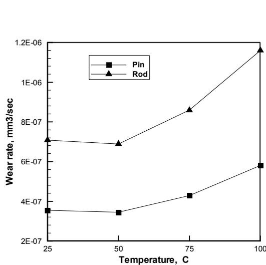
Figure 3. Effect of lubricant temperature on cycle averaged wear rate
