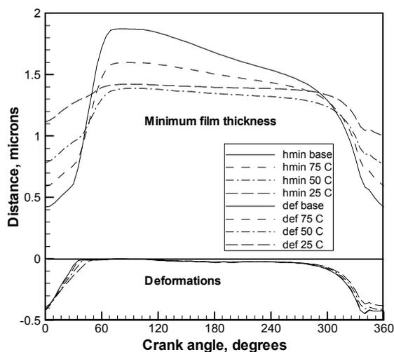
Figure 1. Effect of lubricant temperature on minimum film thickness and maximum deformation
