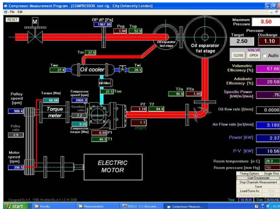
Figure 1 Layout of the compressor test rig
