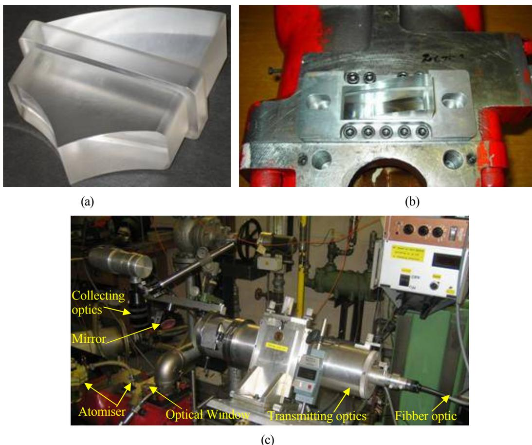
**Figure 2** Optical compressor set up: (a) transparent window and its internal profile; (b) modified compressor with transparent window near the discharge; (c) LDV optical set up of transmitting and collecting optics.
