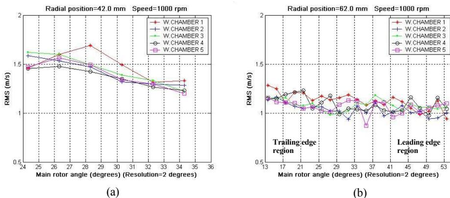
**Figure 6** Working chamber to chamber angular variation of axial rms velocity at two radial positions of  $r=42$  and  $62$  mm and at a rotational speed of 1000 rpm.
