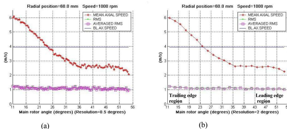
**Figure 4** Angular variation of axial mean and rms velocities across the working chamber for two angle-windows resolution of 0.5 and 2 degrees at a radial position of  $r=60$  mm and at a rotational speed of 1000 rpm.
