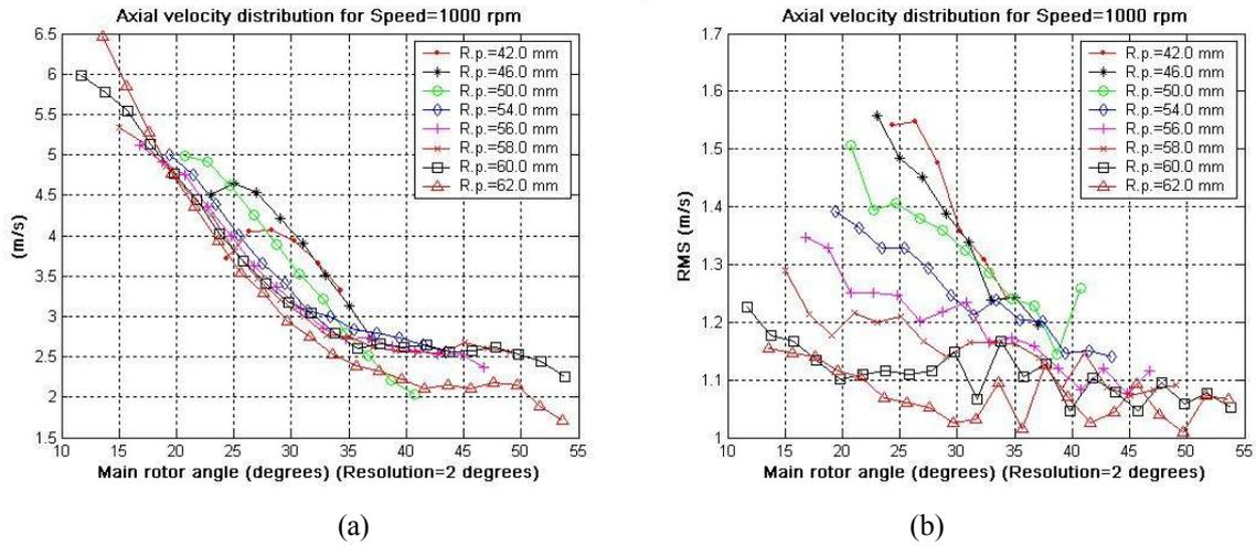
Figure 8 Axial mean and turbulent flow development across the working chamber at different radial positions of  $r=60$  mm and for a rotational speed of 1000 rpm.
