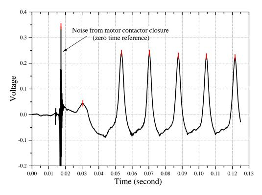
Figure 2 The once-per-turn timing signals. The rotational angle between two adjacent timing signals is 360°.
