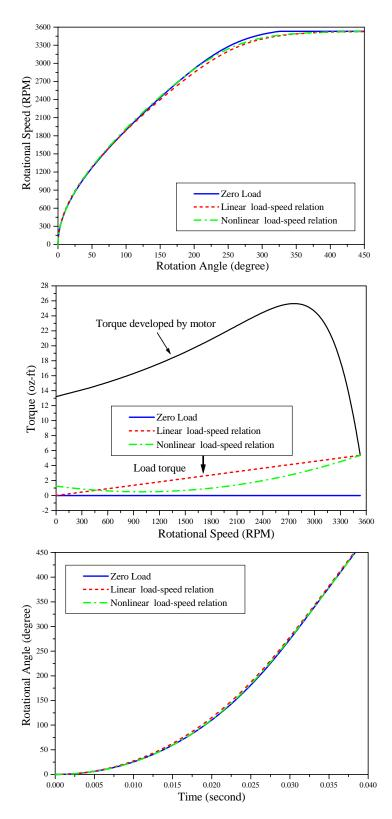
Figure 3 Startup calculation results using the motor speed-torque curve in Figure 1 and the timing signals in Figure 2 and Table 1. Three different functions of load torque  $T_L$  versus rotational speed V are used in the calculations. (1 oz-ft = 0.08474 Newton-Meter, RPM = Revolutions Per Minute).
