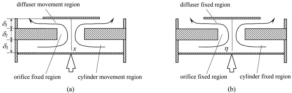
Figure 2: Coordinate system transformation: a) physical domain; b) computational domain.
