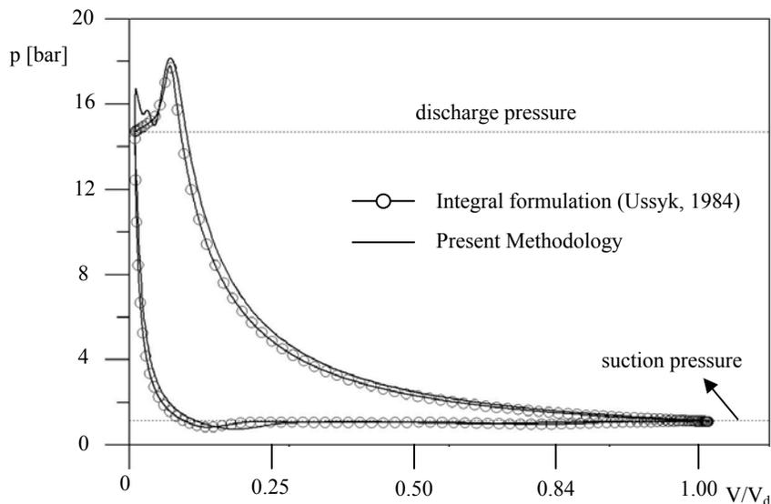
Figure 5: Comparison between integral and differential formulations.
