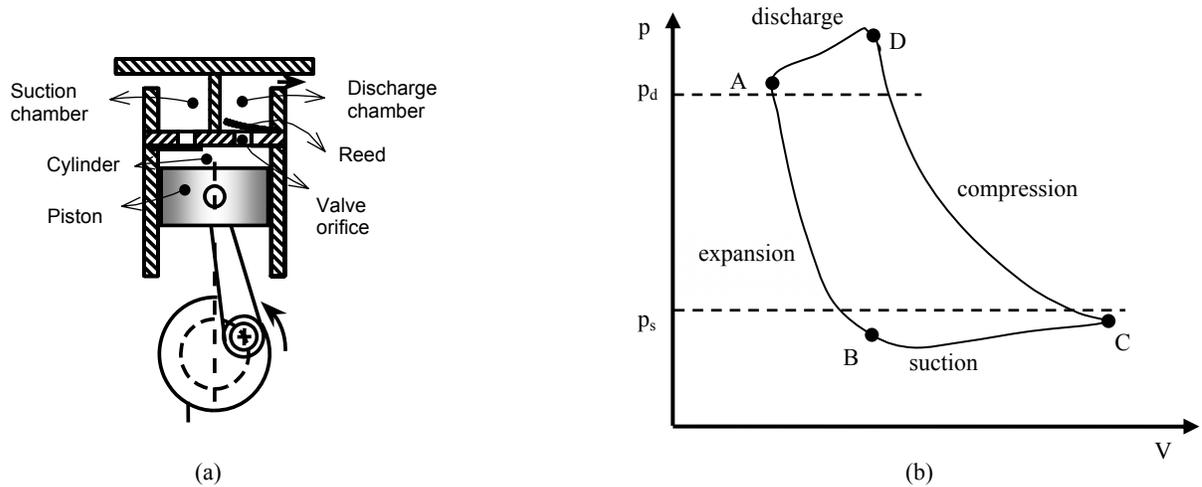
Figure 1: Schematic diagram of a reciprocating compressor and its indicator diagram.
