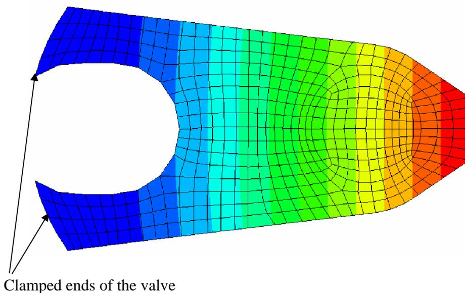
Figure 3: The FEM model of reed valve
