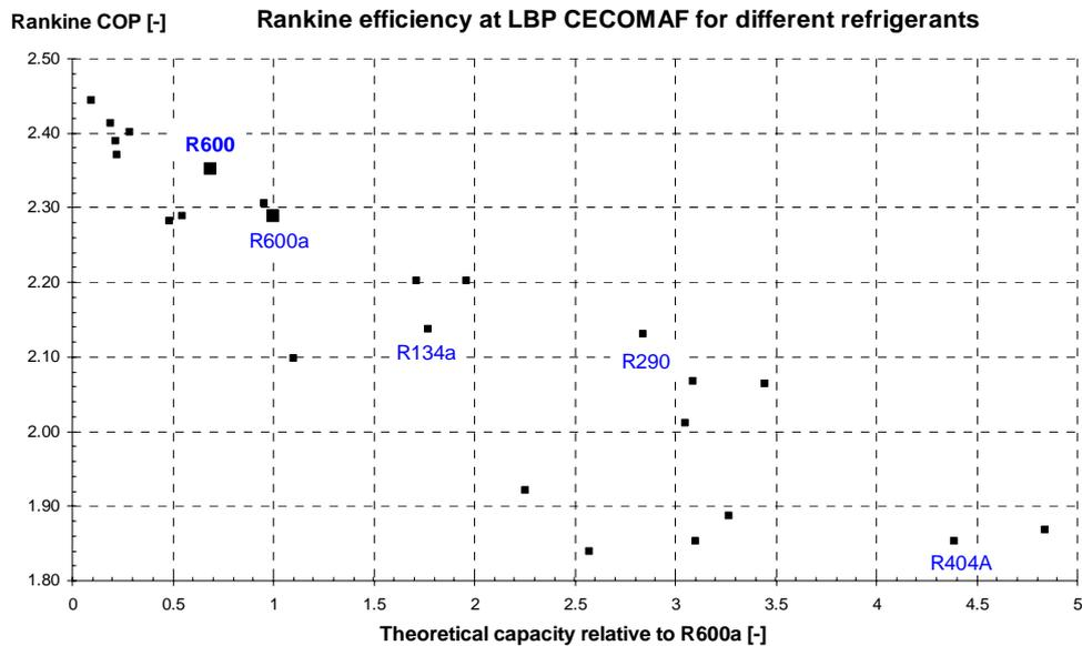
Figure 1: Comparison of theoretical capacity and COP for a reverse Rankine cycle without any losses.
