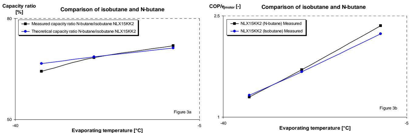
Figure 3a: Capacity ratio NLX15KK2 isobutane/N-butane. 3b: Comparison of  $\text{COP}/\eta_{\text{motor}}$ . Measured at  $55^\circ\text{C}$  condensing temperature. Average of 7 compressors.
