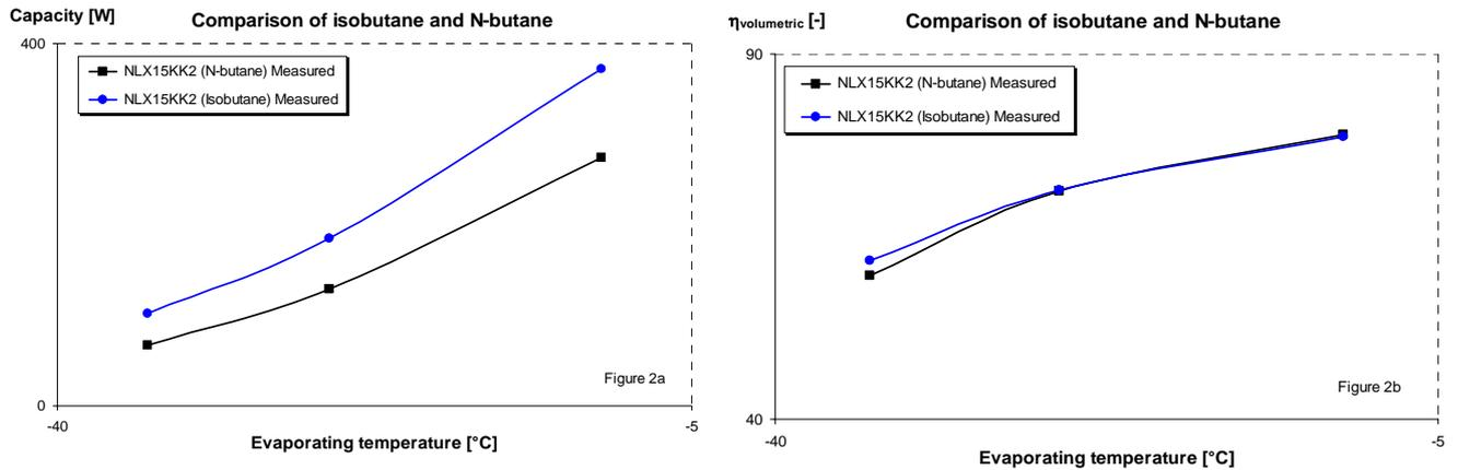
Figure 2a: Capacity for NLX15KK2 using isobutane and N-butane. Figure 2b: Comparison of volumetric efficiency. Measured at  $55^\circ\text{C}$  condensing temperature. Average of 7 compressors.
