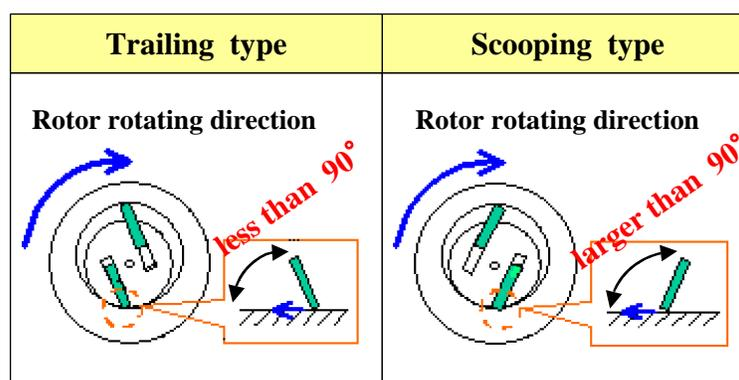
Figure 3: Two types of the vane sliding form
