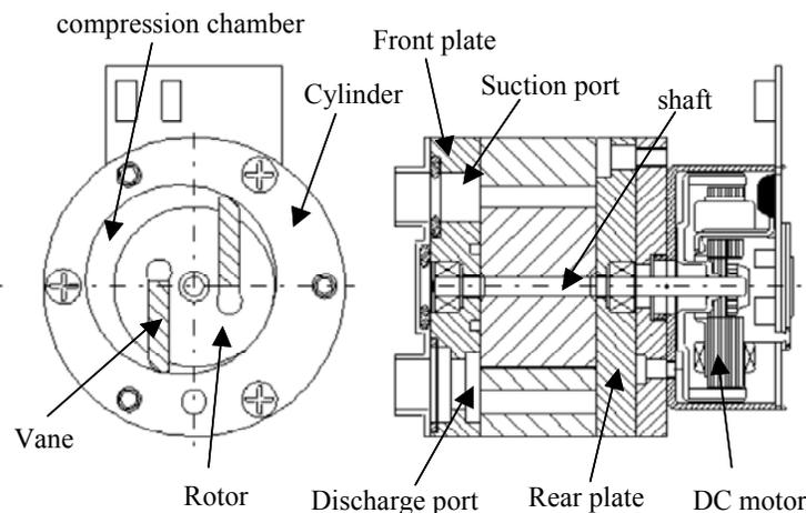
Figure 1: Basic structure of the air pump
