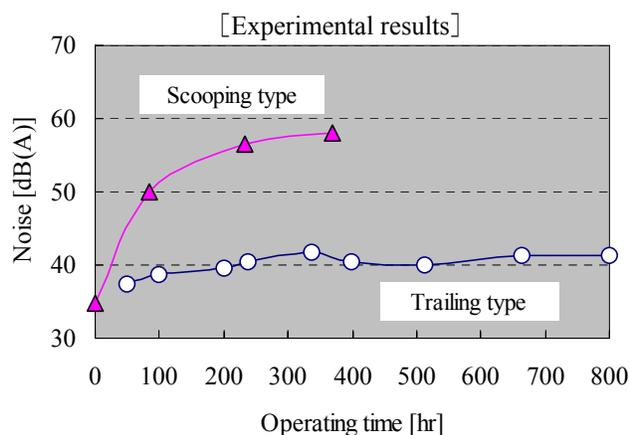
Figure 7: Noise change characteristics of the air pump
