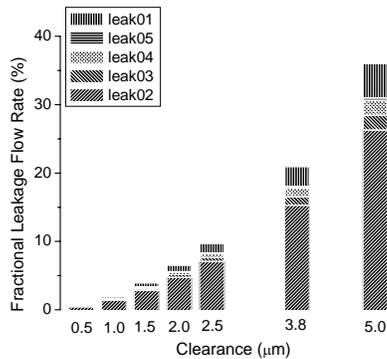
Figure 10: Effect of clearance on leakage.
