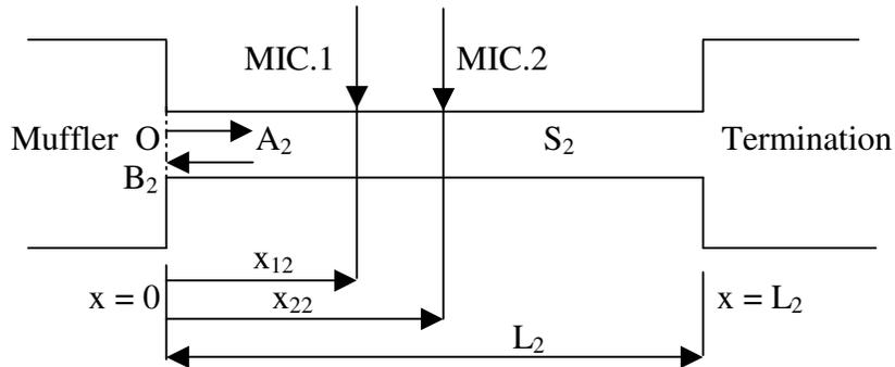
Fig. 2: Location of microphones in the outlet duct
