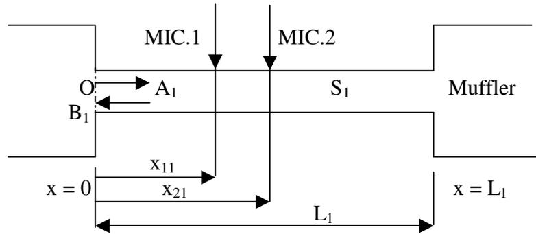
Fig. 1: Location of microphones in the inlet duct
