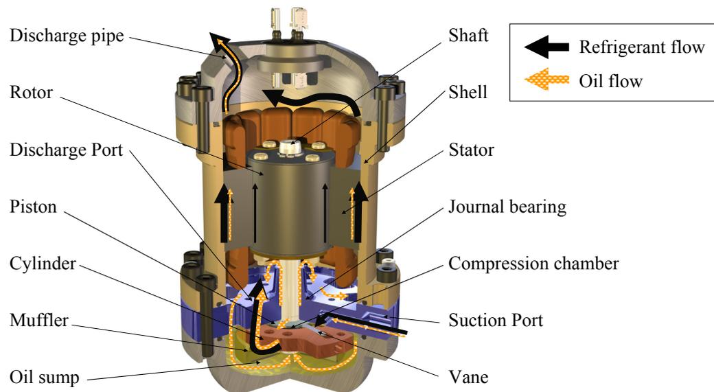
Figure 1: Cross-section of CO<sub>2</sub> rolling piston compressor
