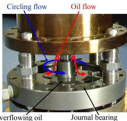
Figure 9: Flow of journal bearing lubrication oil
