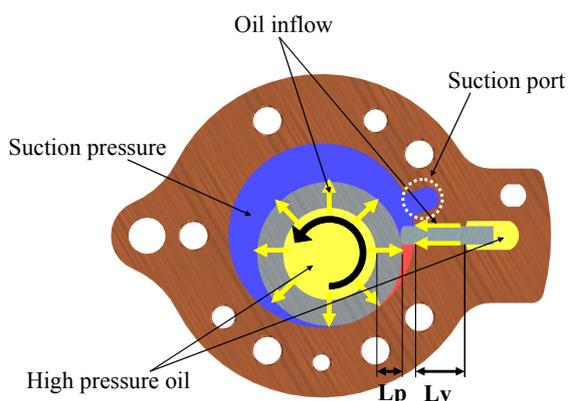
Figure 2: Oil inflow path to compression chamber
