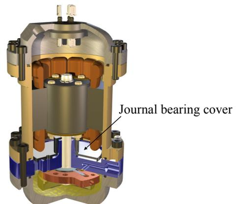
Figure 10: Cross-section of CO<sub>2</sub> rolling piston compressor with journal bearing cover
