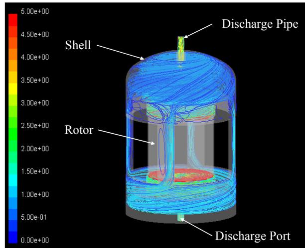
Figure 6: Analysis results of CO<sub>2</sub> flow in shell
