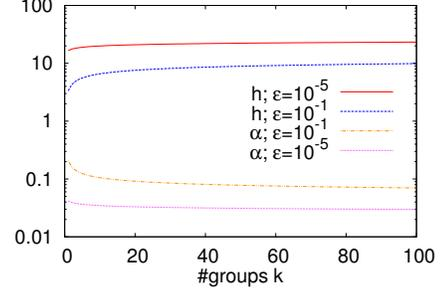
**Figure 4: Dimensioning SVBF: lower bound on #hash functions  $h$ , and upper bound on load  $\alpha = n/m$ , as function of #delay groups  $k$ , for two target  $p_{\text{CF}}$  classification failure rates  $\varepsilon = 10^{-1}$  and  $10^{-5}$ .**
