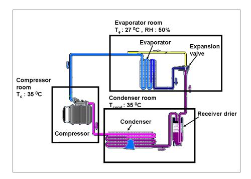
Figure 4: Block diagram of system calorimeter test rig.
