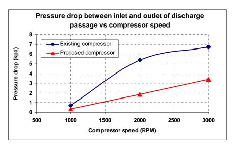
Figure 3: CFD results - Pressure drop vs rpm for existing and proposed compressor
