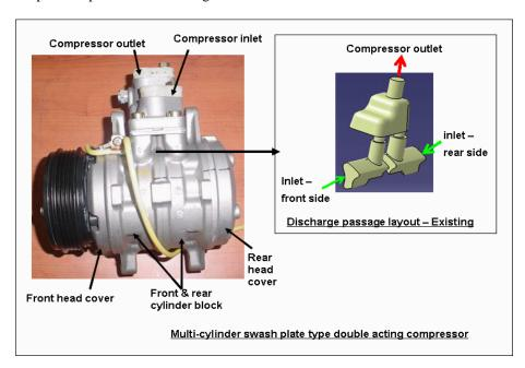
Figure 1: Existing compressor with its discharge passage layout
