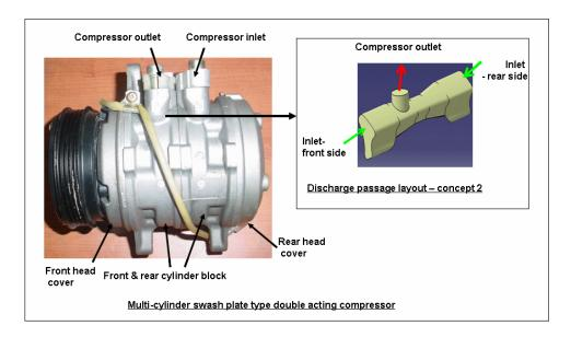
Figure 2: Proposed compressor with its discharge passage layout
