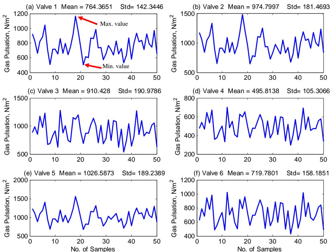
Figure 2: (a)-(f) Gas pulsation in the suction manifold without change in radius at various valve locations.
