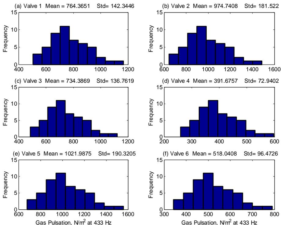
Figure 3: (a)-(f) Gas pulsation in the suction manifold without change in radius at various valve locations.
