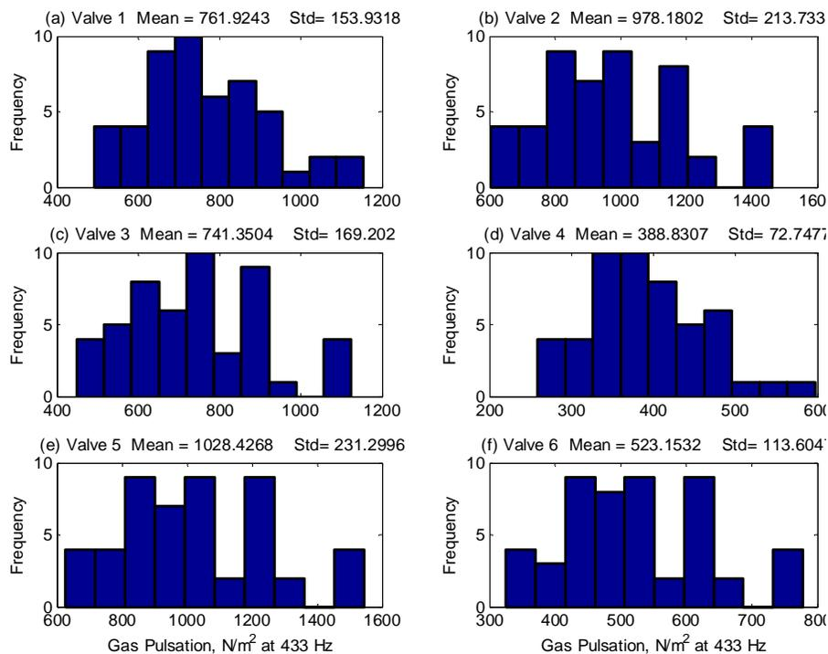
Figure 4: (a)-(f) Gas pulsation in the suction manifold with change in radius at various valve locations.
