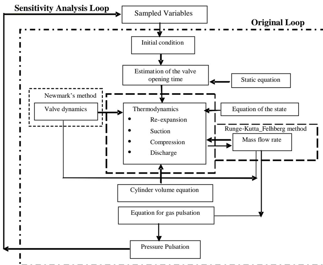
Figure 1: Simulation model showing sensitivity analysis loop outside the original loop.
