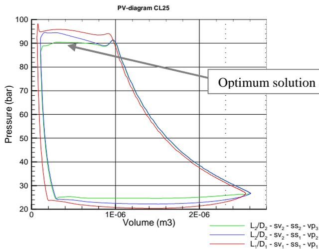
Figure 3. PV diagram CL25 – different configurations
