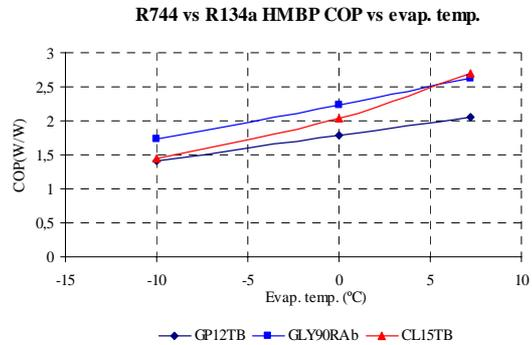
Figure 8. R744 vs R134a HMBP COP vs. evap. temperature
