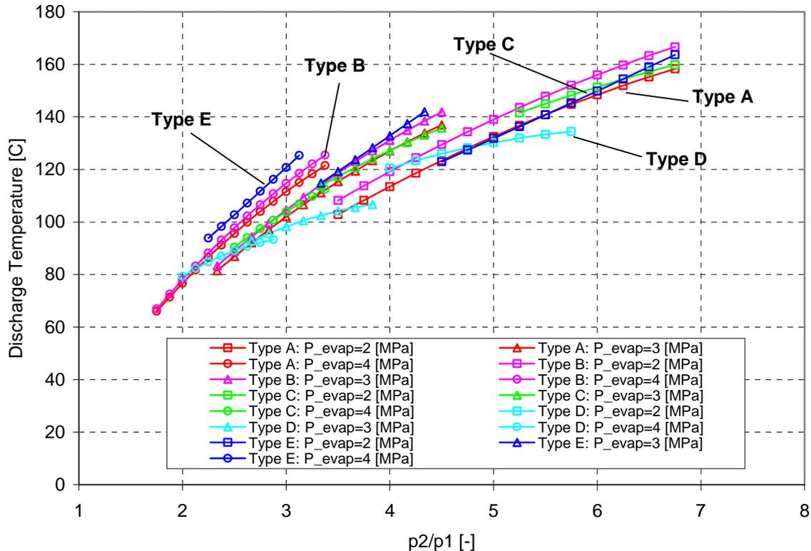
Figure 6: Discharge temperature for evaporation pressures of 2, 3, and 4 MPa versus pressure ratio
