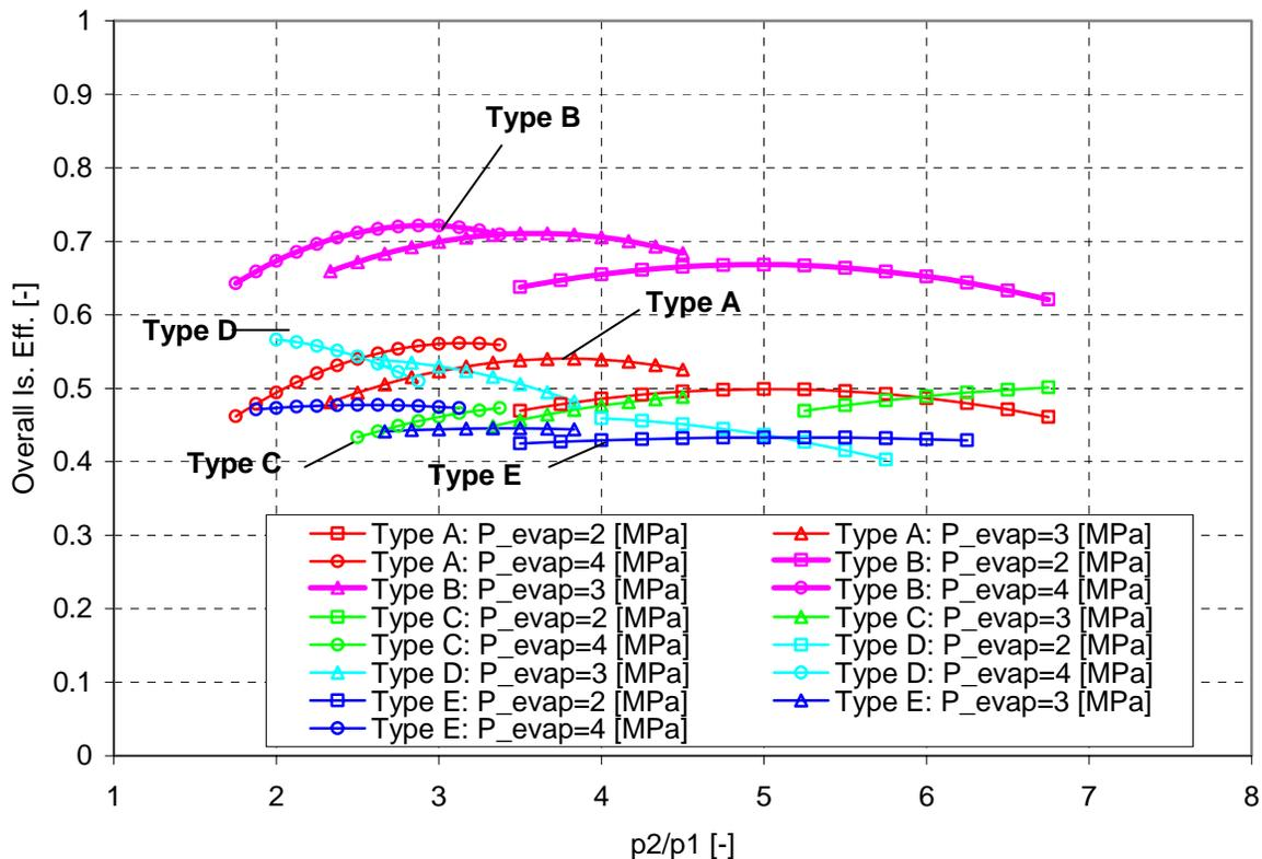
*Figure 5: Overall isentropic efficiency for evaporation pressures of 2, 3, and 4 MPa versus pressure ratio*
