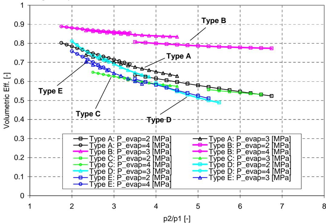
Figure 4: Volumetric efficiency for evaporation pressures of 2, 3, and 4 MPa versus pressure ratio
