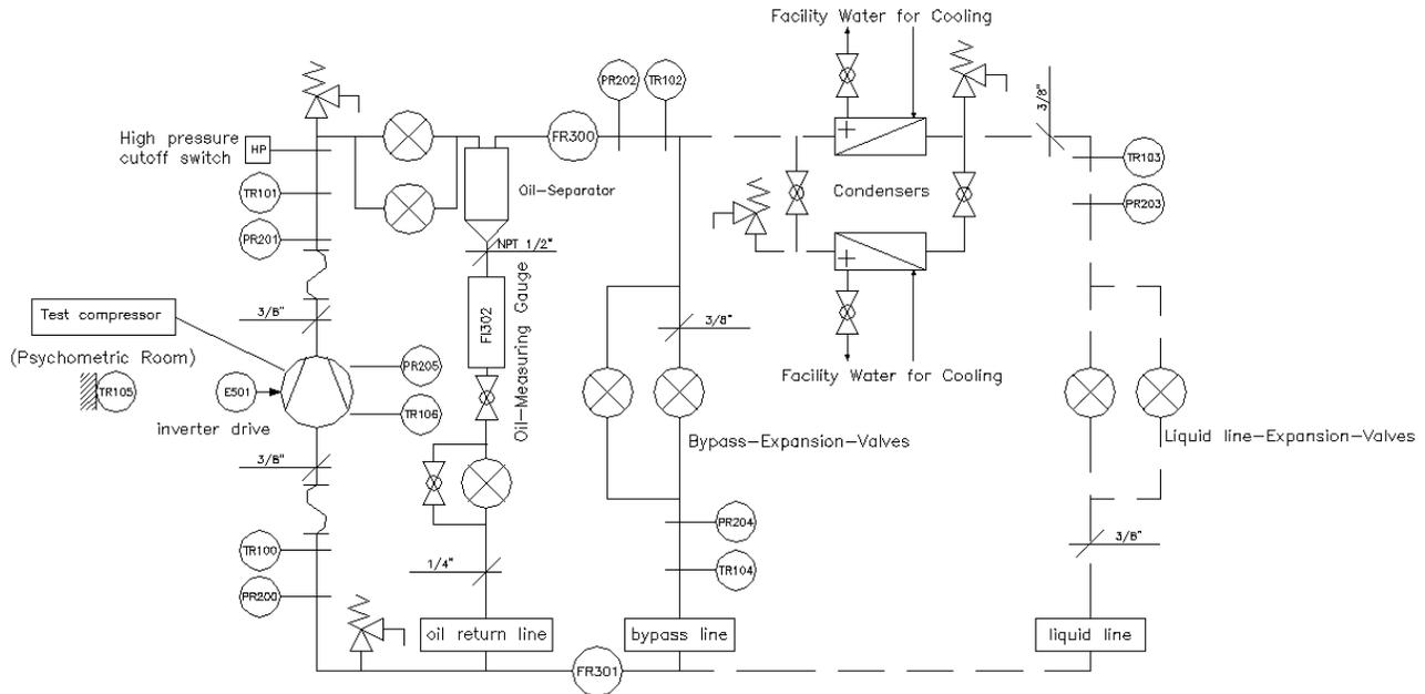
Figure 2: Load stand schematic with instrumentation
