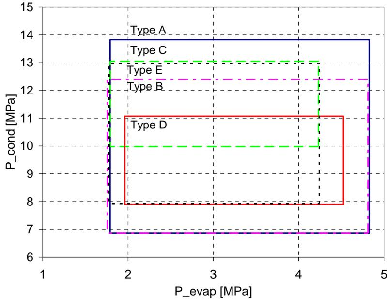
Figure 3: Superposition of all tested pressure fields of compressors A to E
