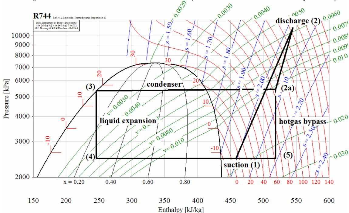
Figure 1: Compressor load stand cycle in P-h-diagram
