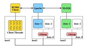
Fig. 7. RUBiS experiment setup
