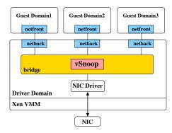
Fig. 4. Xen I/O architecture and vSnoop on Xen
