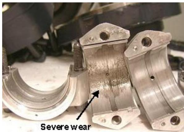
Figure 14: Example of severe crank bearing wear on shell bearings from connecting rod of CO<sub>2</sub> HPWH compressor.
