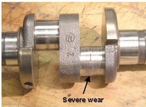
Figure 13: Example of severe crank journal wear on crankshaft of CO<sub>2</sub> HPWH compressor.
