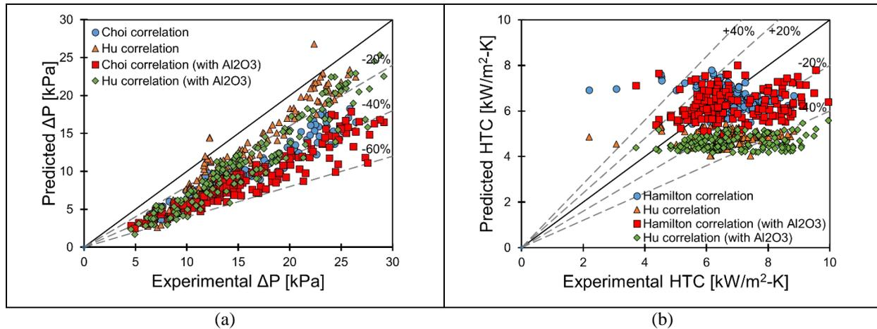
**Figure 1:** Comparison of predicted (a) pressure drops ( $\Delta P$ ) and (b) heat transfer coefficients (HTC) vs. experimental data (data were presented in a companion paper by Deokar *et al.* (2016))
