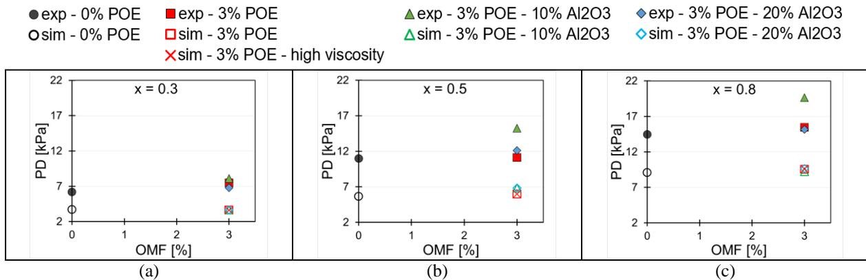
**Figure 3:** Pressure drop for (a) low quality, (b) medium quality and (c) high quality of different refrigerant/lubricant mixtures at test conditions of  $250 \text{ kg/m}^2\text{-s}$  and  $12 \text{ W/m}^2$  (the simulation data in this figure were obtained from application of Choi *et al.* (1999) correlation)
