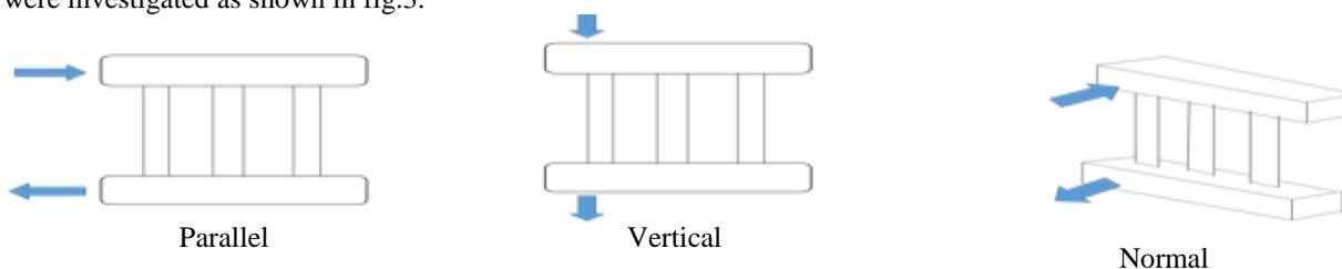
**Fig 3. Flow Inlet Configurations**
