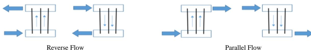
Fig 1. Different methods of tube inlet/outlet configurations.
