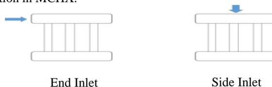
**Fig 5. End Inlet and Side Inlet Configurations**
