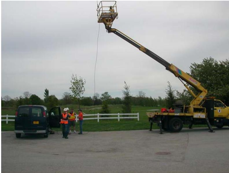
**Figure 16:** Remote radio equipment in van and antenna as hoisted by INDOT boom truck at test site number 3.
