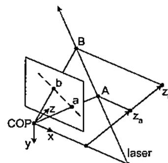
Figure 4 Epipolar line and triangulation.
