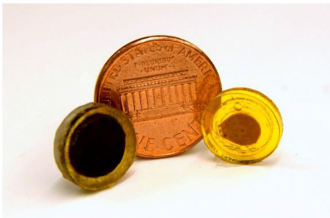
Figure 5. Optical photograph of fabricated prototype (device without ferrofluid on right and device with ferrofluid on left).
