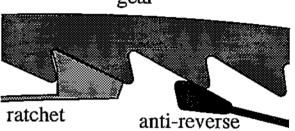
Figure 1: Torsional ratcheting actuator: (top) SEM image courtesy of Sandia National Laboratories Intelligent Micromachine Initiative www.mems.sandia.gov; (bottom) Detail of CAD model.
