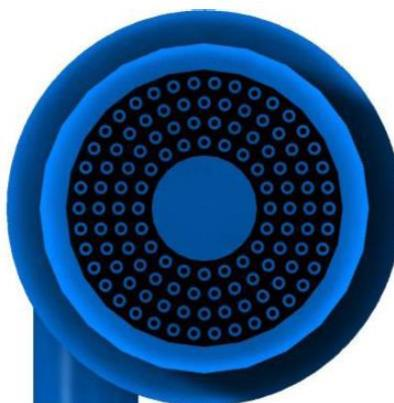
**Figure 2:** Cross section of the 116 tubes mini-channel heat exchanger. The internal diameter is 0.5 mm; the shell side hydraulic diameter is 1.8 mm.
