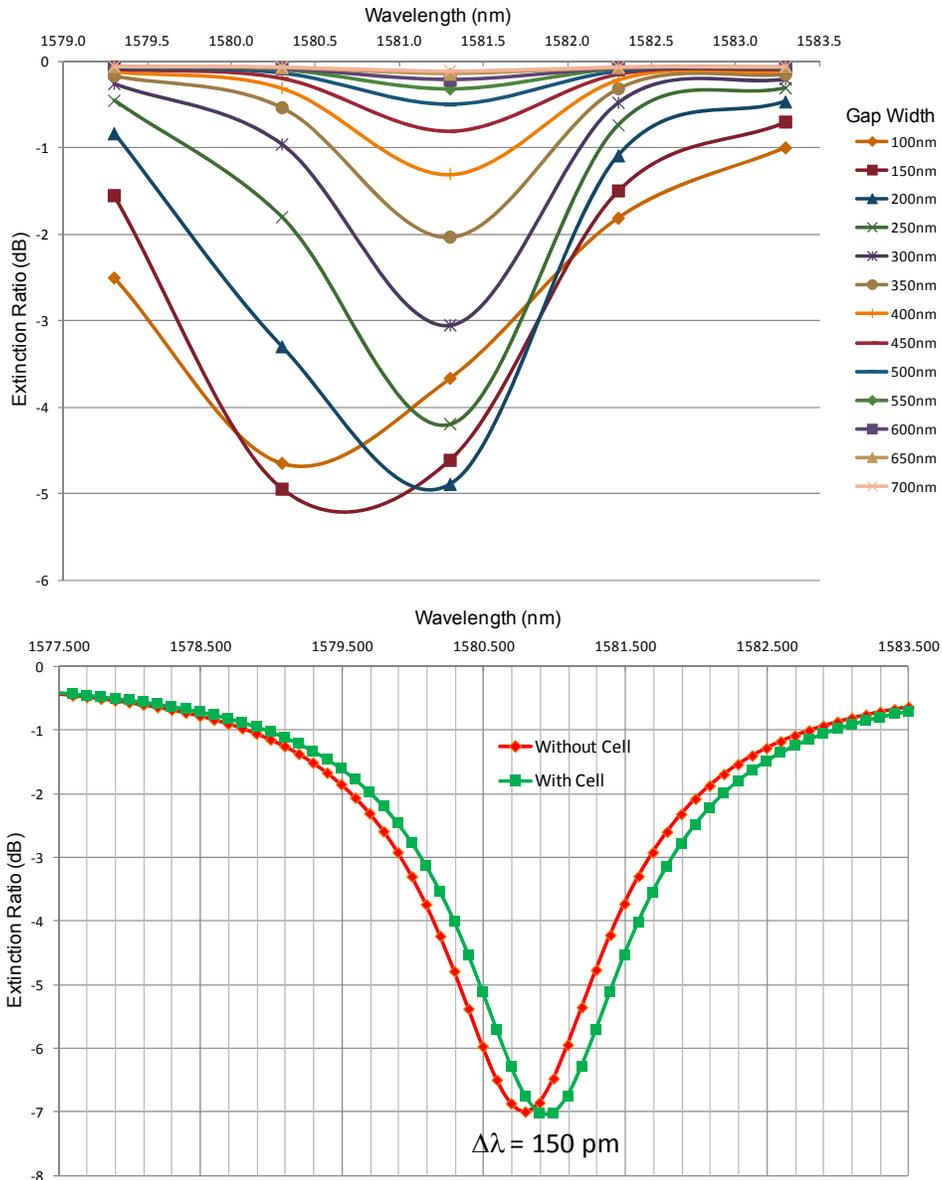
Figure 5: (a, top) Parameter sweep optimization of ring to waveguide coupling gap; (b, bottom) transmission spectra of ring resonator with and without a cell present
